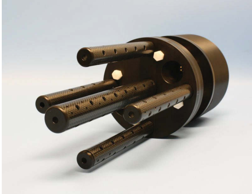
Figure 12: The mini-LRAB acoustic homing receiver. This system integrates the receiving array and processing in a water-proof package for use in small-to-medium size AUVs.
