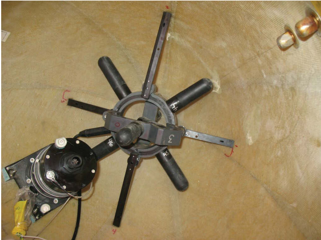
Figure 11: The Long-Range Acoustic Bearing receiver in the nose cone of a large AUV.
