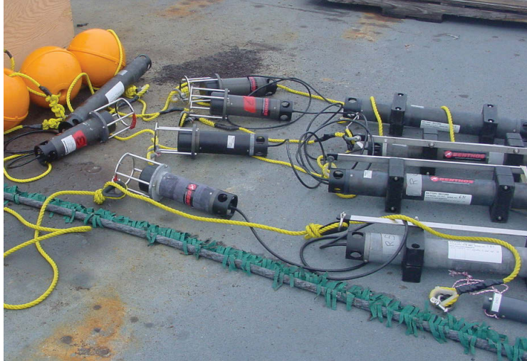
Figure 15: Teledyne modems with separate electronics and battery canisters are ready for deployment. The transducer must be in contact with the sea water and must be located to have an acoustically transparent field of view. Generally, in AUV applications, the transducer is mounted on the dorsal or ventral surfaces.
