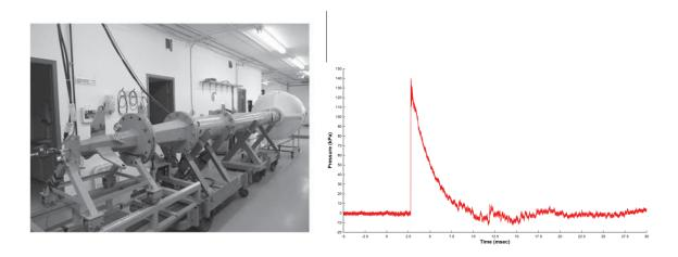
Figure 1.(a) DRDC Suffield Research Centre Blast Simulator. (b) Representative of a pressuretime history trace for the incident shockwave.
