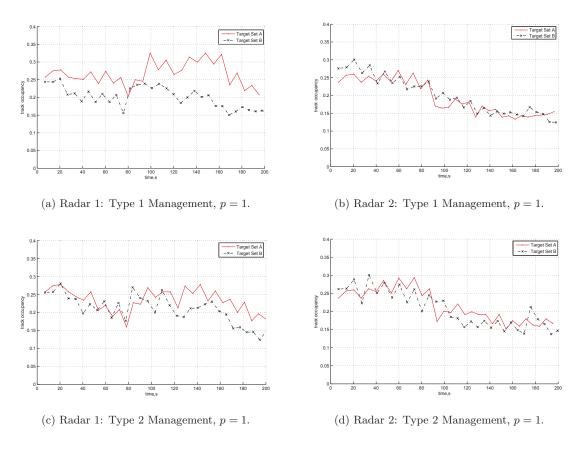
Figure 14: Comparison of track occupancy for Target Set A and Target Set B.
