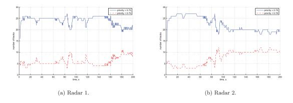
Figure 8: Number of high-priority and low-priority tracks for Type 1 Management for Target Set A.
