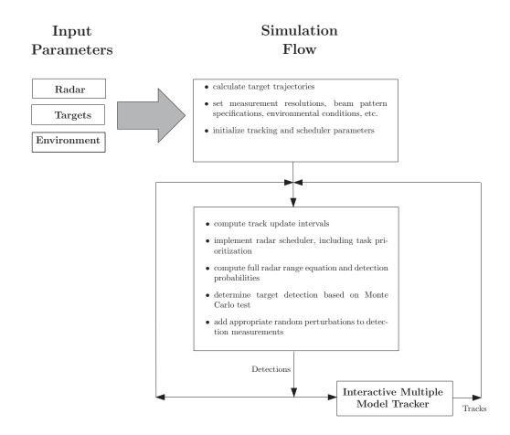
Figure 6: High-level overview of the simulation mode with IMM tracker in Adapt\_MFR.
