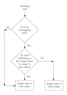
Figure 4: Task assignment algorithm for Type 1 Management.
