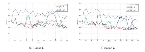
Figure 12: Frame time for the scenario with Target Set A.
