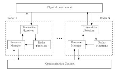
Figure 3: Radar network with distributed management architecture.
