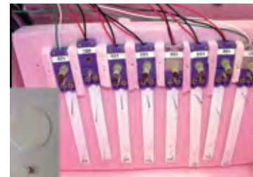
Thermal probe attached to the egg surface (inset), and assembly used to determine the freezing point of several eggs simultaneously.
