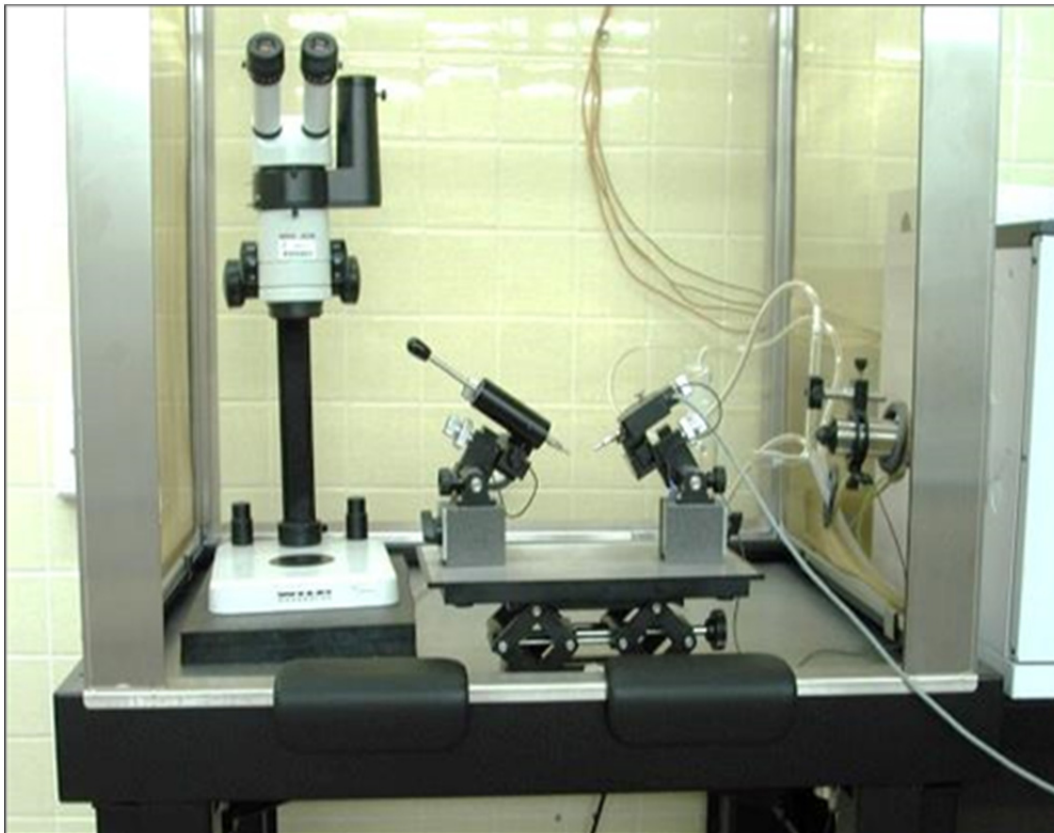
Figure 9. Electroantennogram; device to measure antennal response to volatile stimuli.
