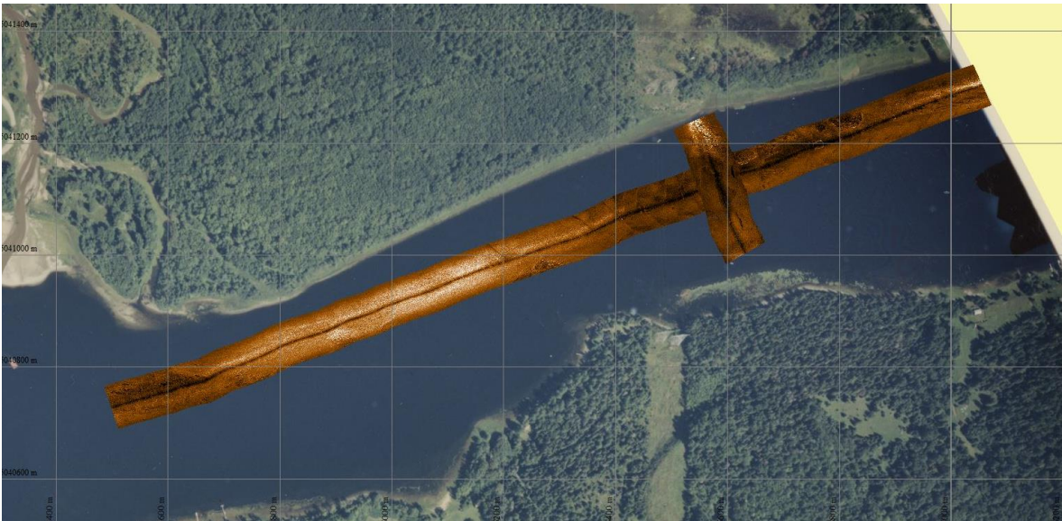
Figure 21. Processing result of a sonar survey line acquired in the flow direction (line 73), and a line acquired across the river (line 81 ), overlaid on an airphoto.
