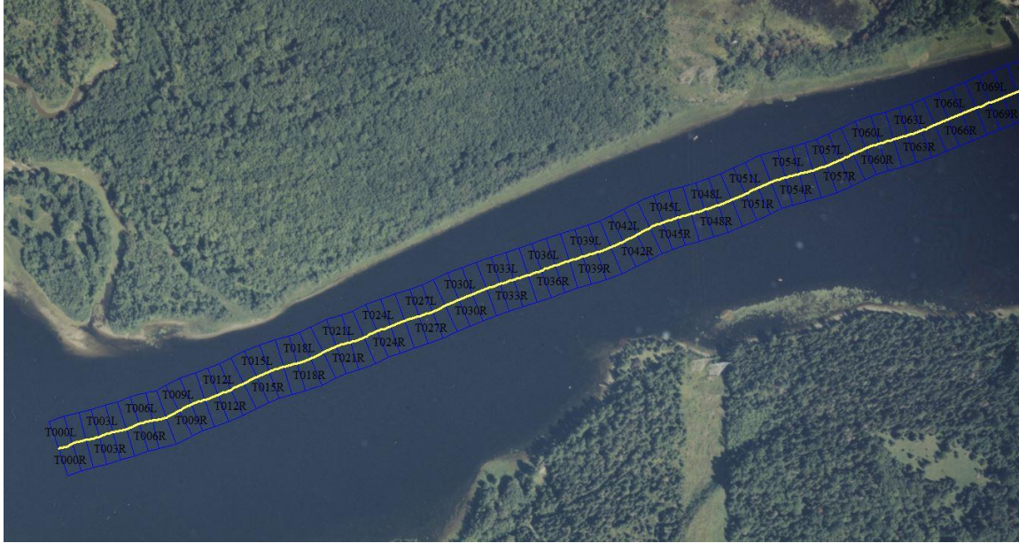
Figure 8. Survey path of a consumer grade side scan sonar overlaid on an air photo.
