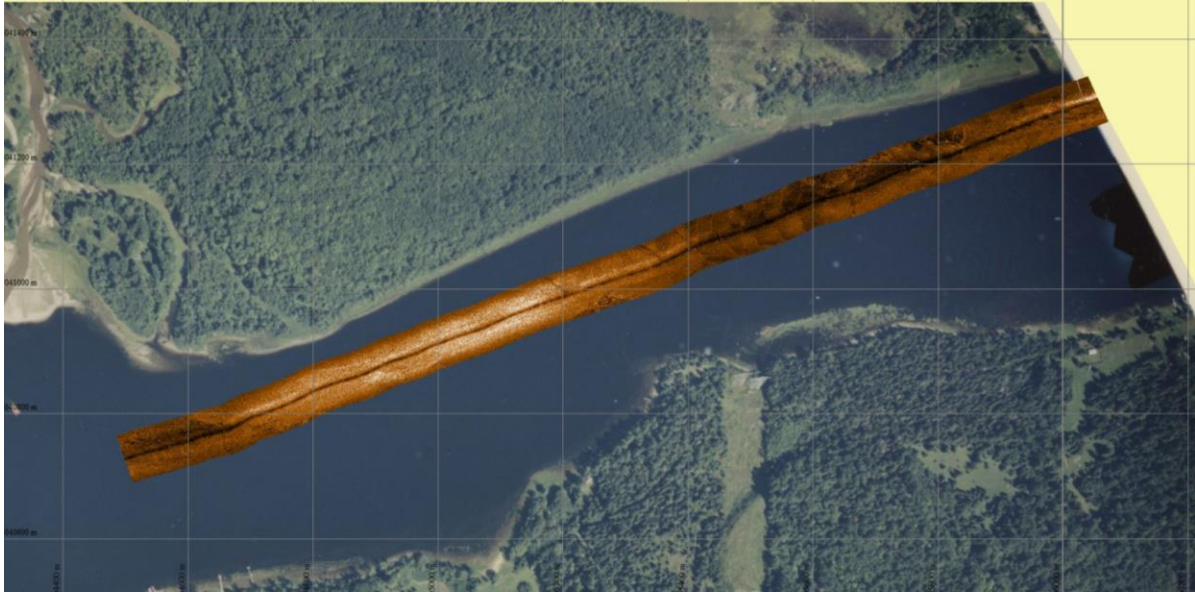
Figure 20. Processing result of a sonar survey line (line 73), overlaid on an airphoto.
