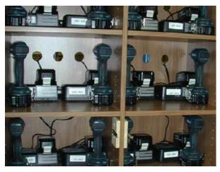
Air drill replacement: Charging station for the cordless tools that replaced the air drills. Estimated annual savings: 36, 832 kWh or \$5,893.
