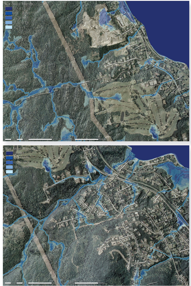
Figure 3: Wet Areas Mapping (WAM) of the community's golf course illustrating flow channels with the greatest likelihood to conduct stormwater during (top) the dry period of late summer, and the wettest weather (bottom) in the spring.
