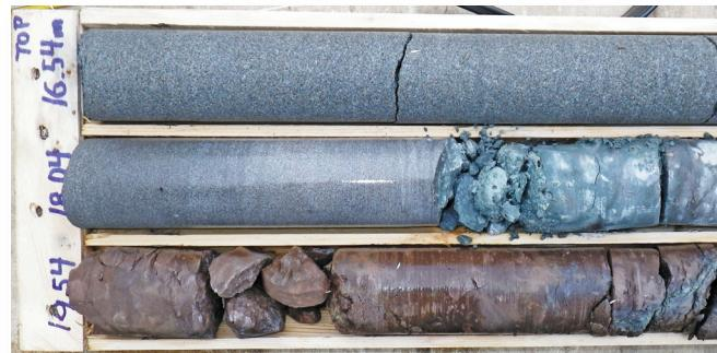
Figure 4: Photo of a drill core used to help understand groundwater movement within the rock, which helps to reveal regions where aquifers may be at risk for salt water intrusion.
