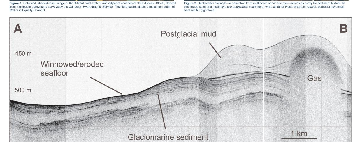
Figure 3. 3.5 kHz seismic reflection profile showing acoustically transparent postglacial mud adjacent to an area of seafloor winnowing and erosion in which acoustically stratified glaciomarine sediments are exposed at the sea floor. Location indicated on the principal map.
