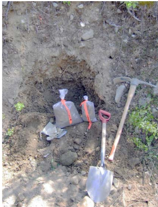
Figure 11: Two till samples from the same site: the large bag (10-15 kg) is for heavy mineral study and the small bag (ca. 3 kg) is for geochemical analyses, physical determinations and archiving (from Plouffe et al., 2009).
