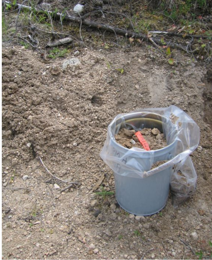
Figure 12: A 20-30 kg till sample in a 20 L pail lined with a plastic bag. Note that the sample number is recorded on the pail and on a tag (flagging tape) inserted in the sample.
