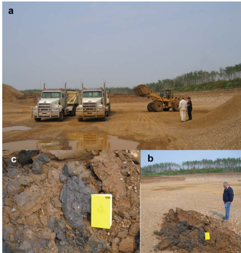
Figure 10: Till sampling at the bottom of an active gravel pit; a) general view of the pit with heavy machinery; b) till dug from the bottom of the pit and deposited by loader on the gravel surface; c) close-up of till.
