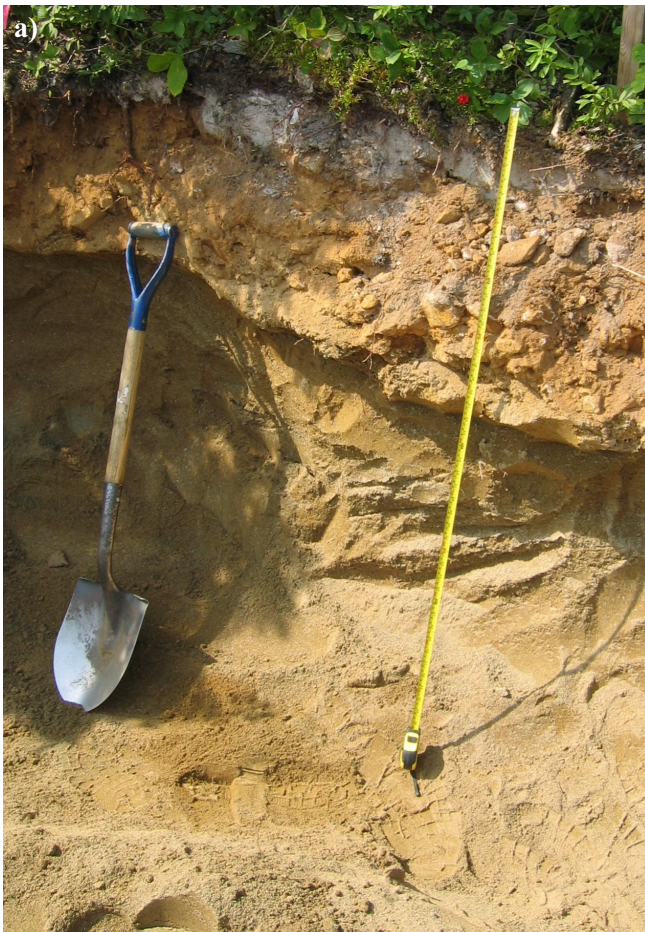
Figure 8. a) Sample site of the unconsolidated weathered Silurian-Devonian granite (grus) used for GSC blank heavy mineral samples; b) close-up view of the blank sample material; and c) close-up view of the 2 to 4 mm fraction of the blank material.
