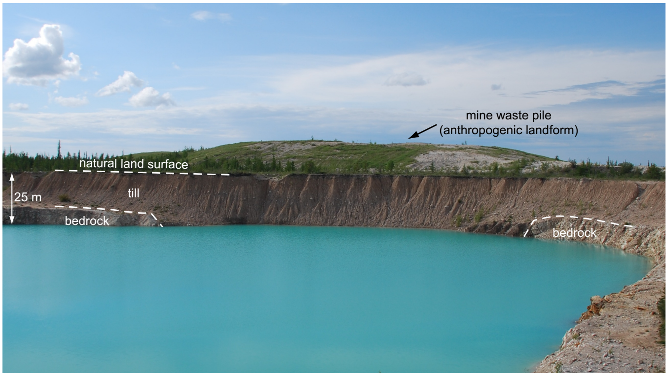
Figure 6. Till sample site in a region heavily disturbed by anthropogenic activity at the old Pine Point Pb-Zn Mississippi Valley-Type mining district, Northwest Territories. Till samples were collected in a former open pit mine, below the original natural land surface (Rice et al., in press) and away from mine waste piles, which consisted of till excavated from the former open pit, mixed with other mine debris.
