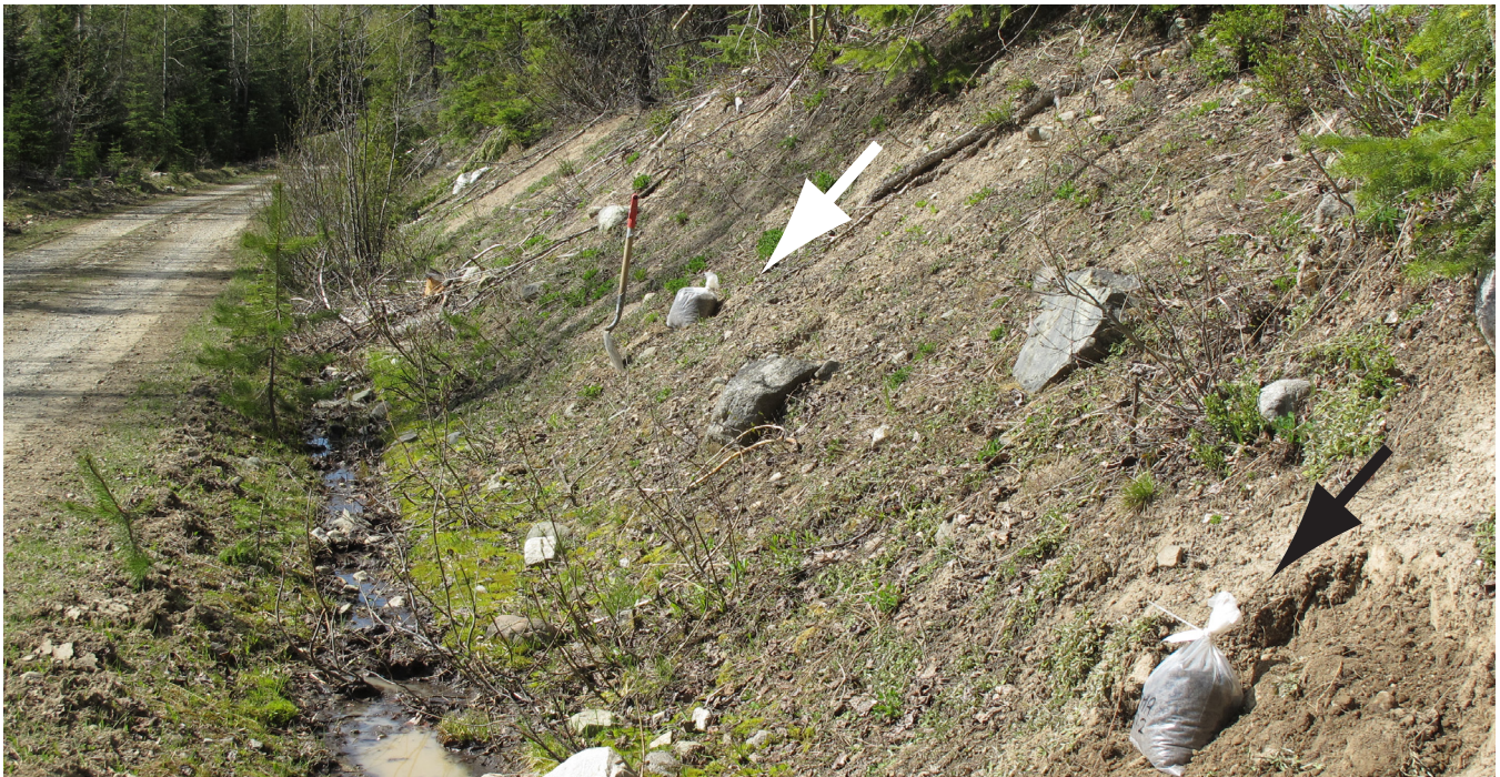
Figure 7. Example of a sampling site from which a routine sample (black arrow) and a field duplicate sample (white arrow) have been collected in the same sedimentary unit and at approximately the same depth.
