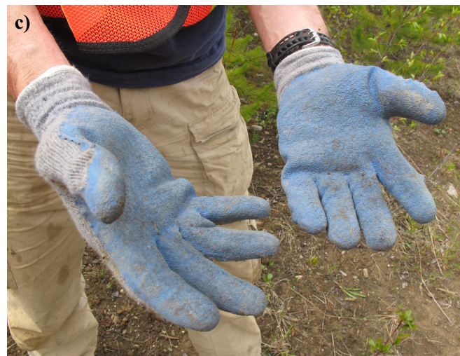
Figures 4. Potential sources of carry-over contamination: (a) a dirty pick with sediment stuck to it after the collection of a sample, and therefore unsuitable for the collection of the next sample; (b) a cleaned pick ready for the collection of a sample; and (c) dirty gloves also represent a potential source of contamination if the subsequent sample is manipulated by hand.
