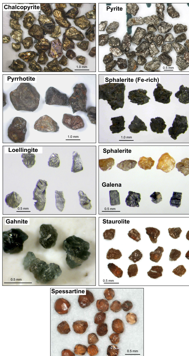
Figure 2. Photographs of selected VMS indicator minerals as they appear in till heavy mineral concentrates around VMS deposits.
