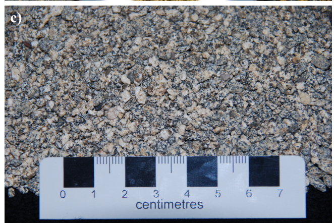
Figure 8. a) Sample site of the unconsolidated weathered Silurian-Devonian granite (grus) used for GSC blank heavy mineral samples; b) close-up view of the blank sample material; and c) close-up view of the 2 to 4 mm fraction of the blank material.
