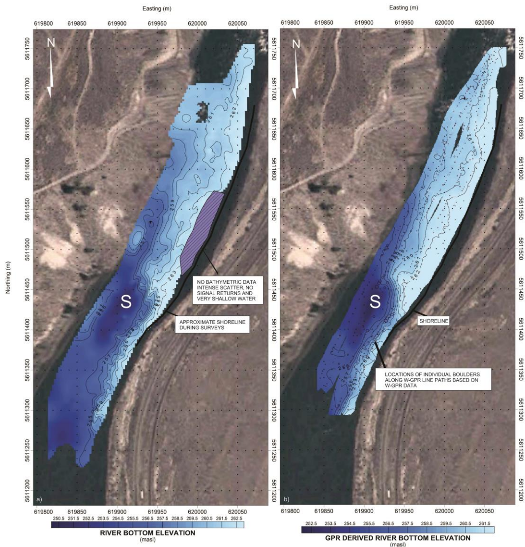
Figure 11 a) Acoustic based river bottom elevation; b) W-GPR river bottom elevation with boulder locations; S – scour pool (after Bauman et al., 2015).
