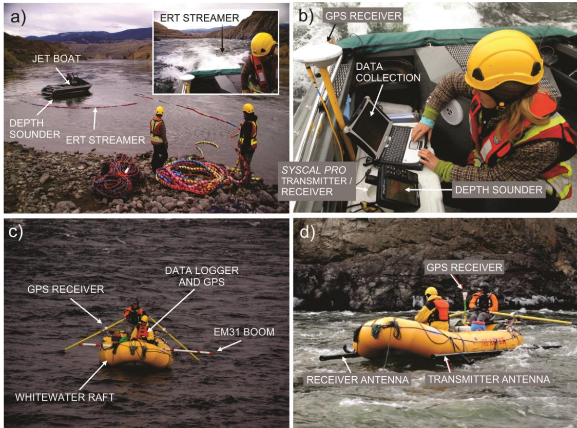
Figure 5 Waterborne geophysics applied over the Thompson River, October-November 2014: a) AB and W-ERT set-up, including jet boat, ERT streamer and depth sounder; b) W-ERT data collection in the jet boat; c) W-EM31 set-up operating mid-channel in Thompson River; d) W-GPR set-up operating along the right channel bank (Bauman et al., 2015).
