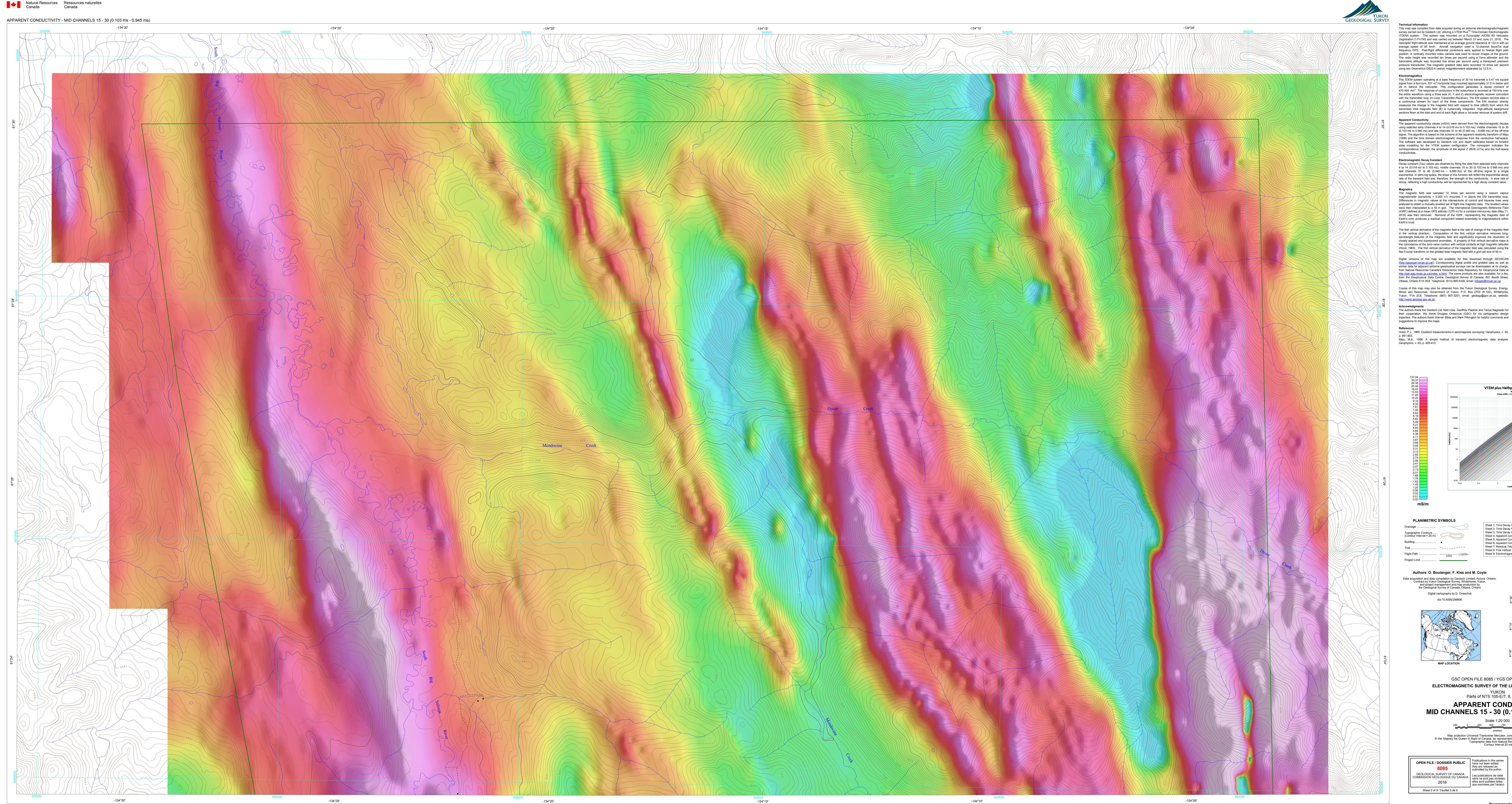
using two Geometrics G822-A cesium magnetometers separated by 12.5 m.
