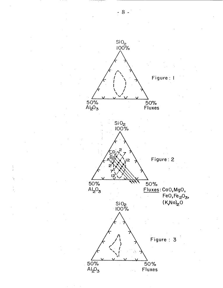
Figures 1-3. Triaxial diagrams showing composition limits of bloating clays
