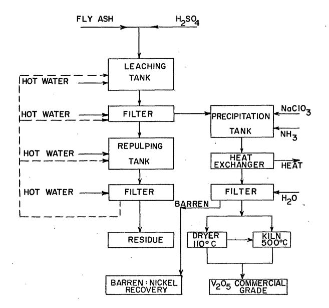
FIGURE I: FLOWSHEET OF A PROCESS FOR THE PREPARATION OF COMMERCIAL GRADE V205 FROM FLY ASH SUBMITTED BY CANADIAN PETROFINA LTD.
