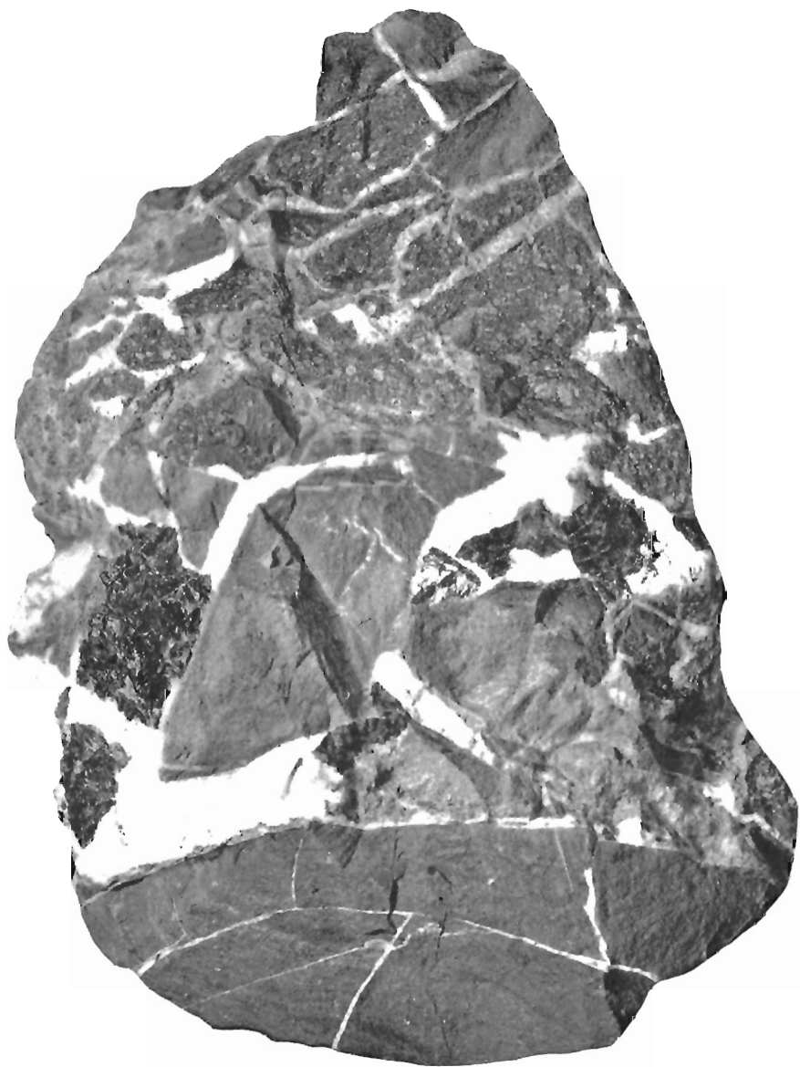
Brecciated shales and limestones, mineralized with sphalerite and quartz. Approximately natural size. (Page 92.)
