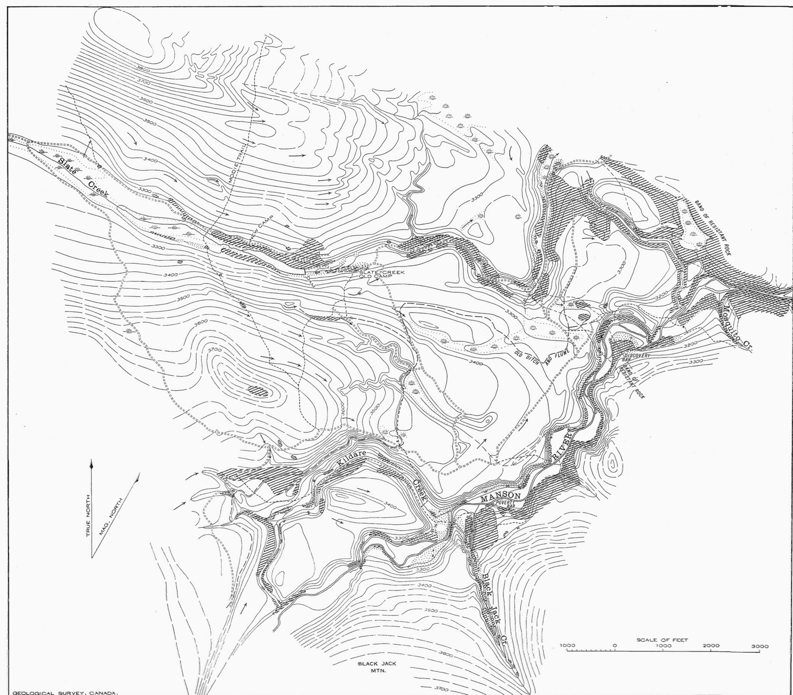
Figure 2. Manson River-Slate Creek area. Areas of old placer workings are shown by pattern of stipple; and areas of bedrock outcrop by diagonal ruling; arrows indicate positions of parts of abandoned stream channels cut in present surface and not clearly indicated by contours.
