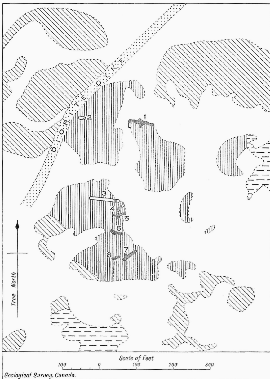
Figure 5. Plan of No. 1 group of ore deposits, Amulet mine, showing pits (Nos. 1 to 8). Ore shown by solid black; outcrops and areas of outcrop of dalmatianite by vertical ruling; rhyolite and rhyolite-breccia (partly altered to dalmatianite) by diagonal ruling; andesite by broken horizontal ruling; and diorite dyke by pattern of stipple.
