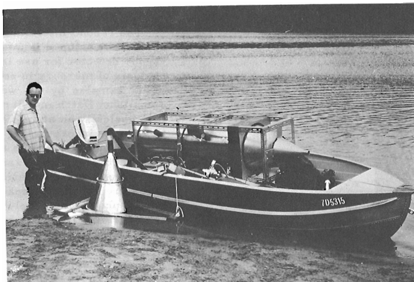
Figure 1. Radon monitoring of lake waters using large ionization chamber. Core attached to the side of the boat collects radon that is released from the water. (GSC photo 202086)
