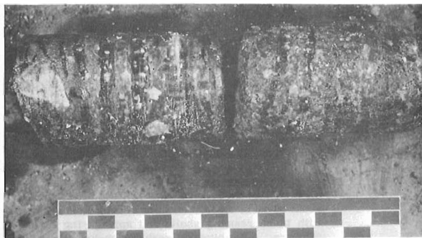
Figure 1b. Weathered granitic bedrock with stratified ice.
