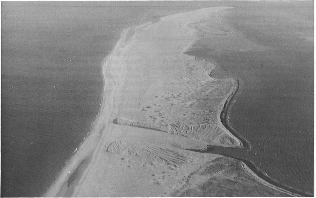
Figure 3. Infilled inlet, Tabusintac, N. B., sediment transport in the littoral zone is from top to bottom.
