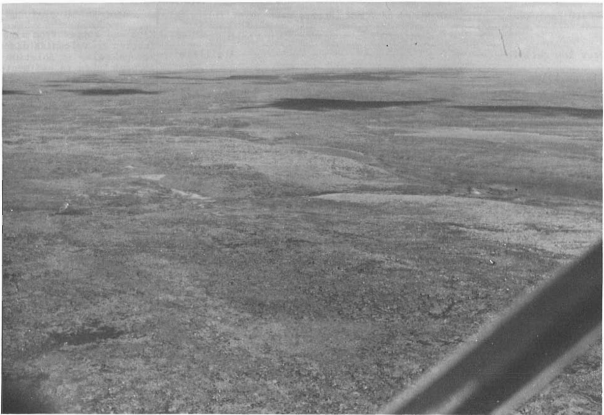
Figure 4. Anomaly Y, photographed facing north from the centre of the area shown in Figure 2, Light coloured ridge of upper siliceous volcanics runs diagonally from right centre of photograph; metasedimentary rocks beyond. Light coloured outcrops in left centre are thickest portion of "B" zone gossans and the underlying altered volcanic rocks.
