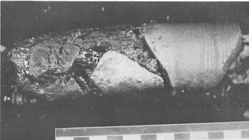
Figure 2c. Clay till with quartzite cobble, visible ice around cobble. Note: Scales at bottom of cores in centimetres.
