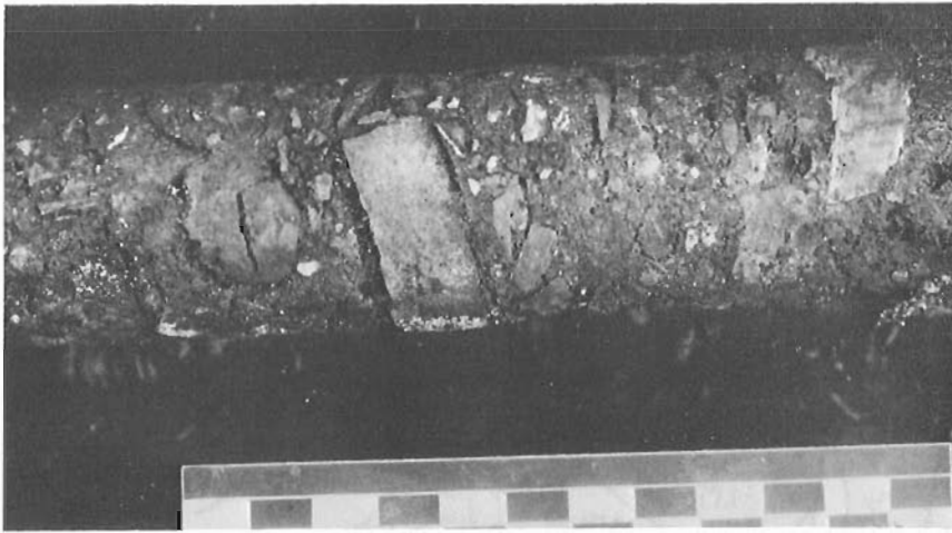
Figure 2a. Till with silty shale and sandstone fragments, low ice content.
