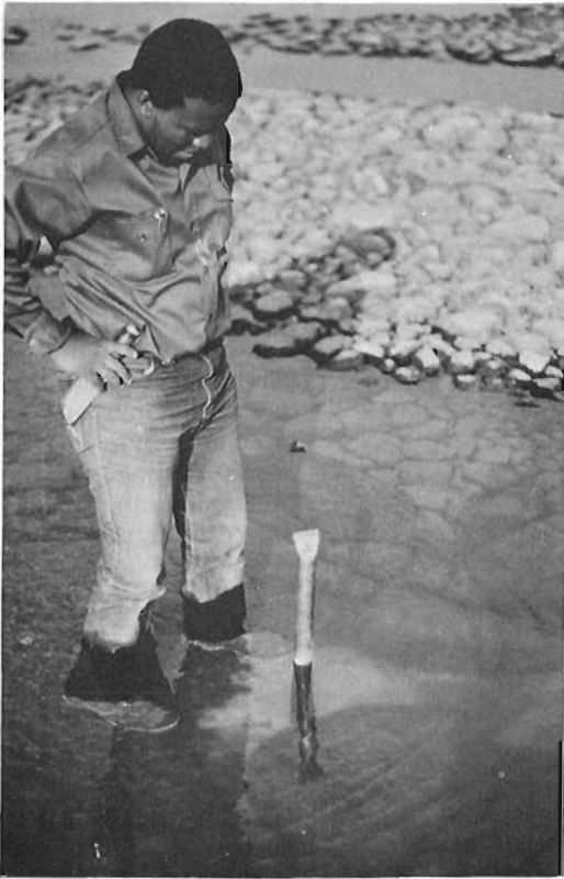
Figure 7. Probing depth to permafrost at edge of island in Kaminak Lake (probe rests on permanently frozen till, 1.5 m below water surface).
