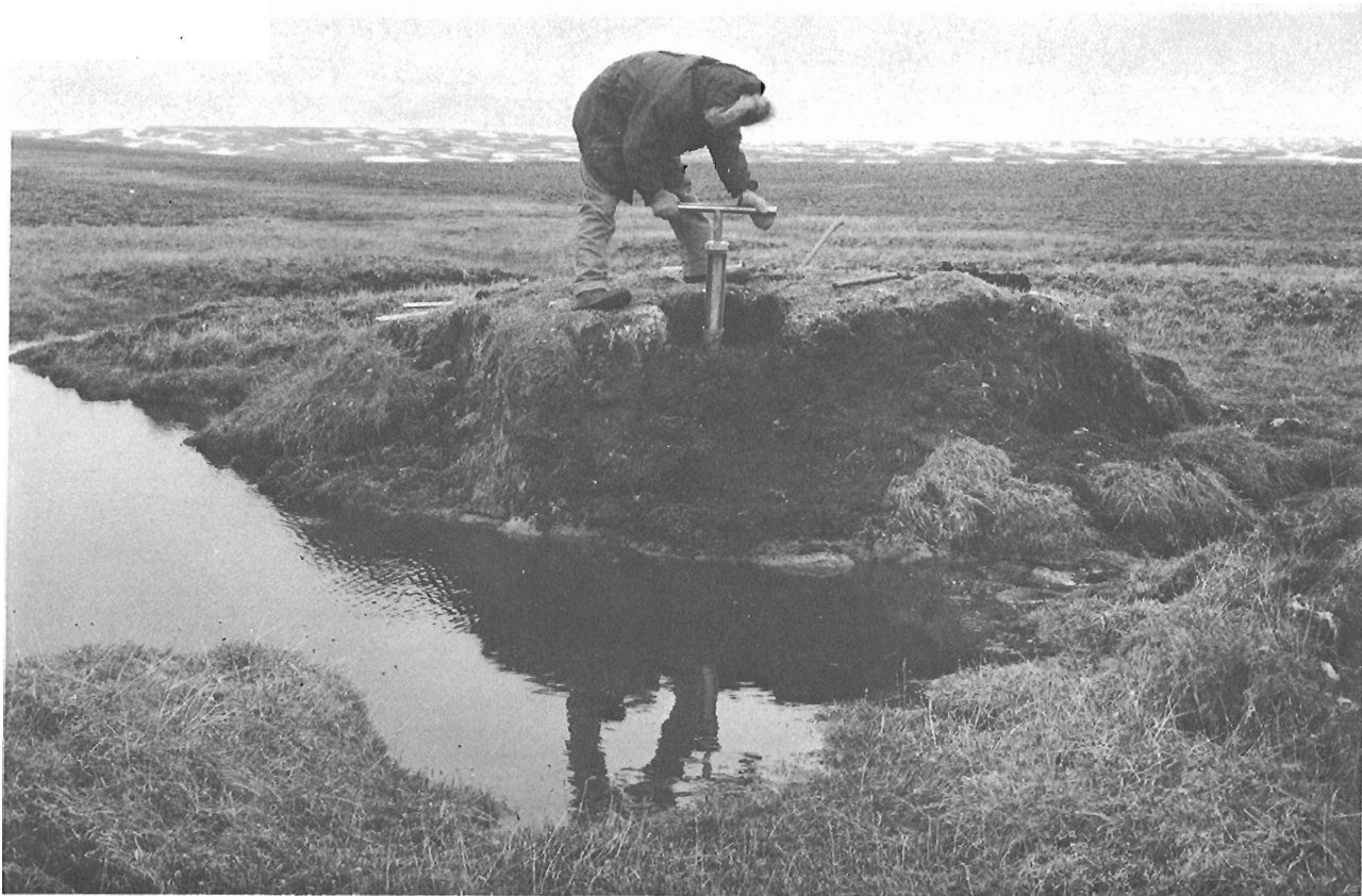
Figure 3. Detail of peat mound on ridge shown in Figure 2. Frozen coring surface was at depth of 21 cm. Open part of core barrel is 35 cm long. Peat at 17-21 cm depth, unfrozen, was 7820 \pm 140 years old (GSC-233). July 2, 1963. GSC photo 202566.
