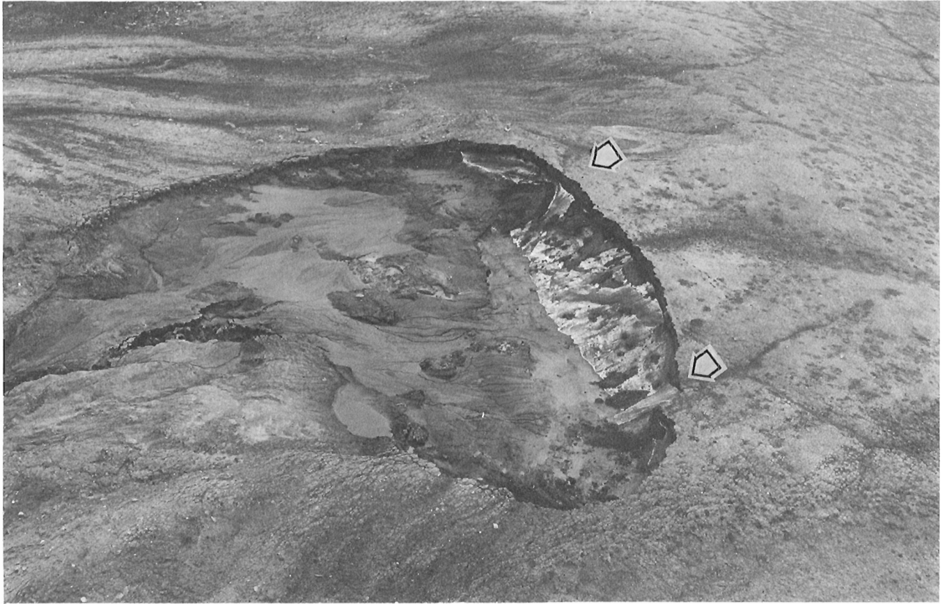
Figure 40. 6. A "thermal cirque" typical of high ice-content clays. Headward retreat was measured at greater than 3.5 m over the summer. These features are a source of significant quantities of fine sediment and are a reliable indicator of high ice-content materials. Similar features at coastal sites showed varying rates of retreat depending on the thickness of the high ice-content material. In the northern part of the island lower rates of retreat probably are associated with colder temperatures. Note the two obvious ice wedges, marked with arrows, in the photograph. The width of the face is approximately 50 m. Photo taken July 9, 1975 on a tributary of Thomsen River.
