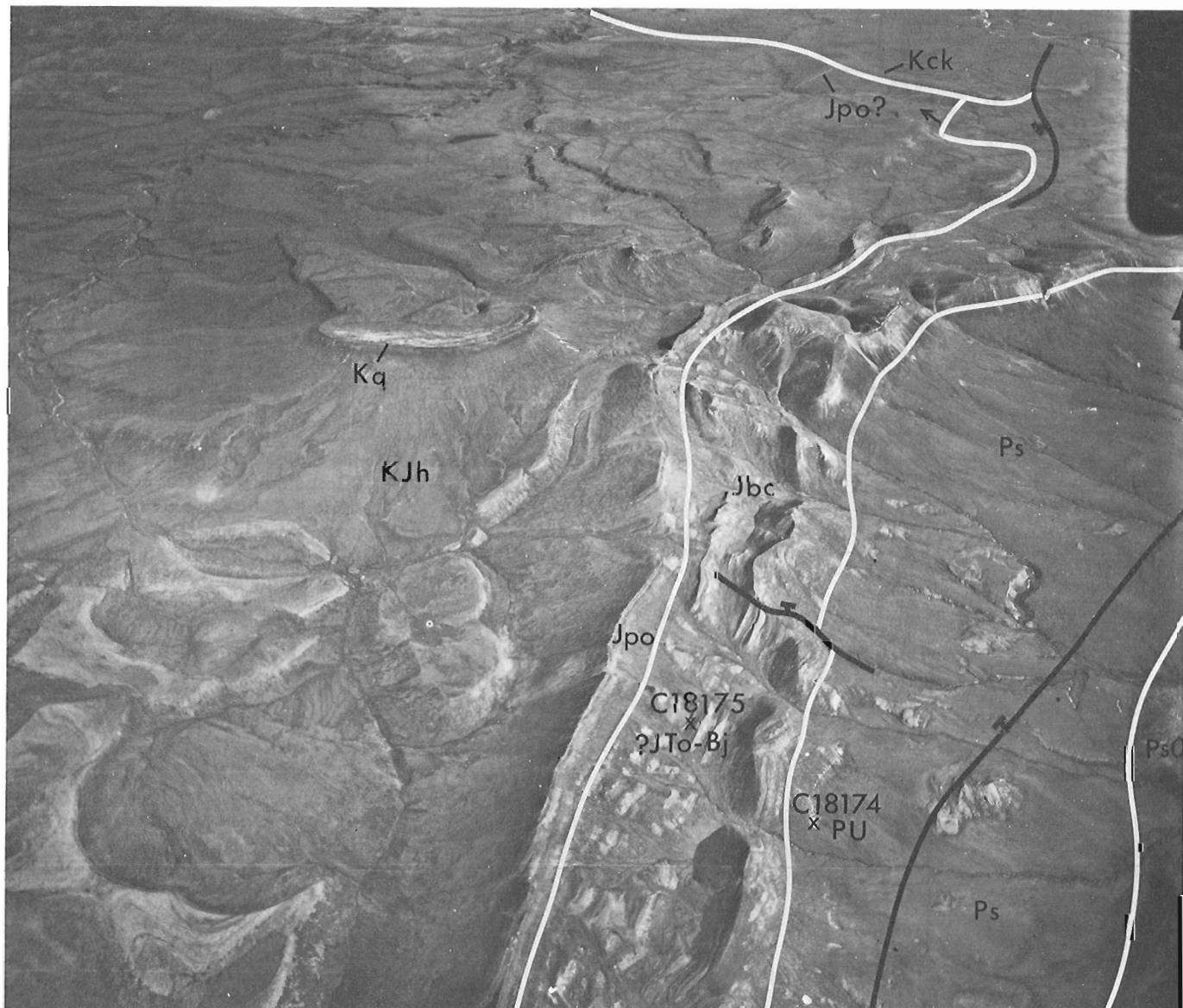
Figure 97. 3. Northwest flank of Cache Creek Uplift showing unconformities 1, between unnamed shales and limestones of the Permian (Ps) and Jurassic (Jbc) Systems; 2, between the Jurassic Bug Creek Formation (Jbc) and unnamed Upper Jurassic sandstones (Jpo); and 3, between the Upper Cretaceous Cuesta Creek Member (Kck) of the Tent Island Formation and deformed Jurassic and Cretaceous rocks. Two GSC fossil localities with ages are also shown. View is to the north-northwest. NAPL Oblique Photograph T-5 22R.
