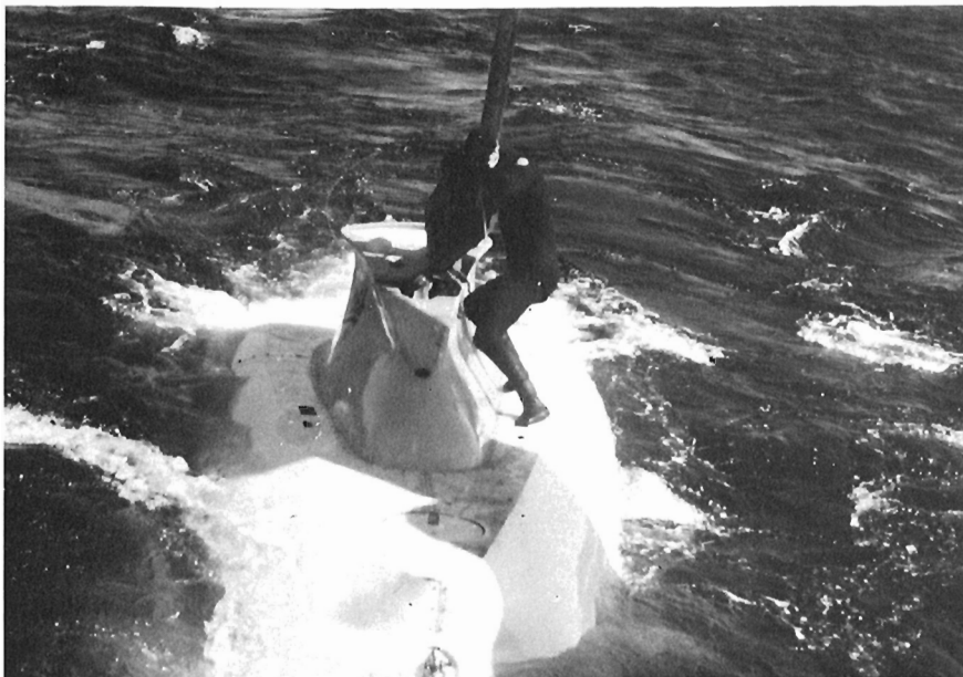
Figure 62. 4 The diver is detaching the hoist cable.
