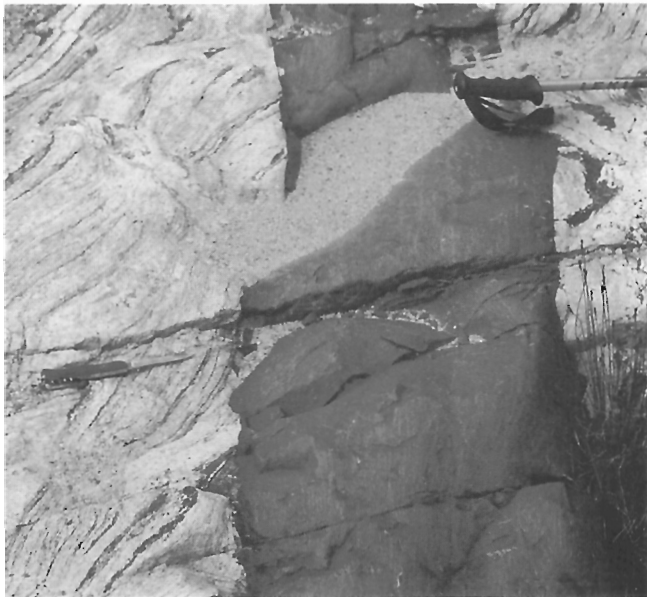
Figure 17. Hairline fracture cutting a Tertiary dyke intruded into gneisses of the Monashee Group at Location 6. Such fractures were the most recent features found at the site.
