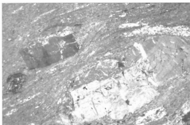
Figure 5. Orvan Brook porphyry. Potassium feldspar phenocrysts plus occasional pseudomorphs after biotite (left centre of the photomicrograph).
