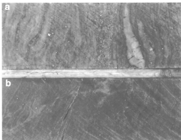
Figure 5. Photograph of drill core (DDH 122-7) showing intensely altered footwall sedimentary rocks stratigraphically below the inferred Brunswick Horizon (Headway Horizon). a) very silicified sedimentary rocks with minor pyrite veins and disseminations (NF Fm.; 128.3m; LPA-332), b) thin-layered sericitic and chloritic footwall sedimentary rock (PB Fm.; 133.8 m; LPA-333).
