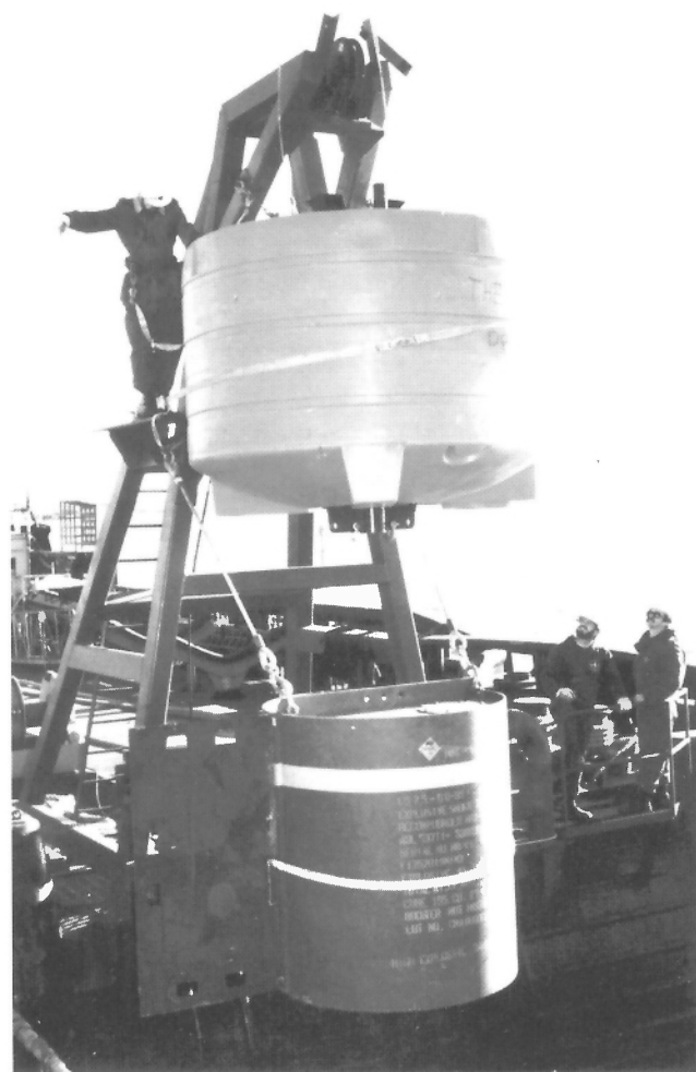
Figure 4. Photo showing the 10 000 lb HBX-1 charge and float prior to deployment.
