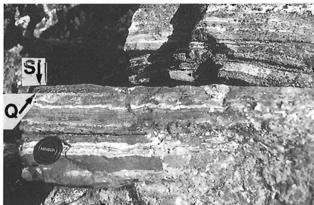
Figure 7. Straight banded magnetite+quartz iron-formation on long limb of a Z-fold. Axial planes of small-scale Z-folds are subparallel to fine quartz ribbons (Q) developed in an attenuated altered (hornblende) silicate iron-formation (S); Discovery zone.
