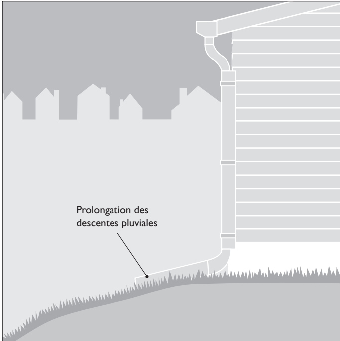
Figure 37 Prolongation des descentes pluviales
