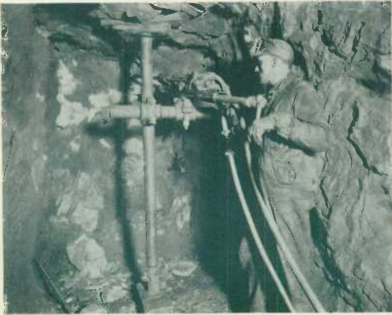
Underground in a Quebec Copper-Sulphur Property.—Drilling by compressed air drill.
