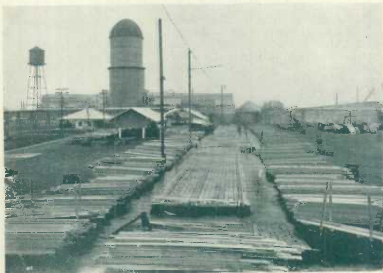
Sorting Tables at a Canadian Sawmill.—The sawn lumber from the mill moves along the conveyor belts and is sorted for length and quality during transmission. Note the trucks drawn up to the sides of the tables to collect the different grades.
