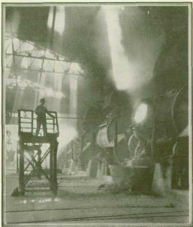
PRODUCTION.—A converter aisle of nickel-copper smelters, with sun-light streaming through the furnace mist and a worker raking off slag.
