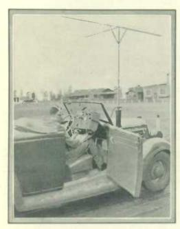
Mobile Radio Telephony Installation in a Light Car as Developed by the Royal Canadian Corps of Signals.
