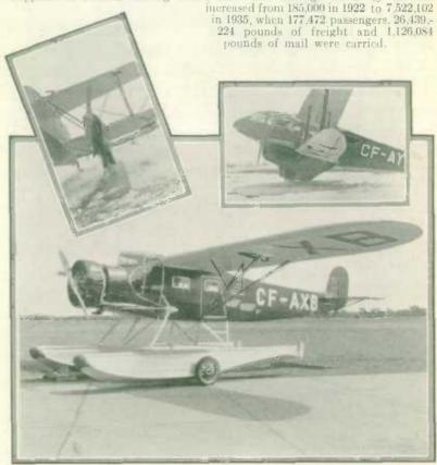
Civil Flying in Canada. The above machine is a recent product of the aircraft industry. It is representative of a type of machine (with either wheels, skis or floats) going into service in the Canadian North. Insets: Front and side views of streamline skis on a transport plane. These skis are the first of their type and were developed by the National Research Council of Canada.
