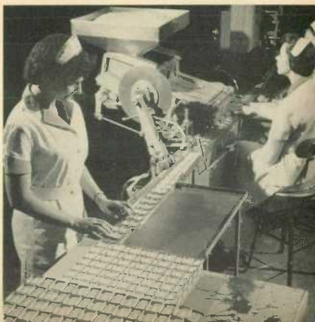
Packaging aspirin tablets—about 6,000 tins are filled in an hour.
