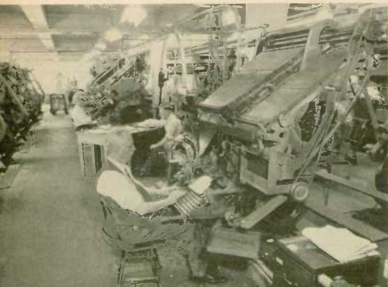
A battery of linotypes — the machines that revolutionized the printing industry nearly seventy years ago. These machines have been refined to the point where they are almost human in their operation. Each costs about $35,000 and devours 2,800 lb. of metal alloy a day.
