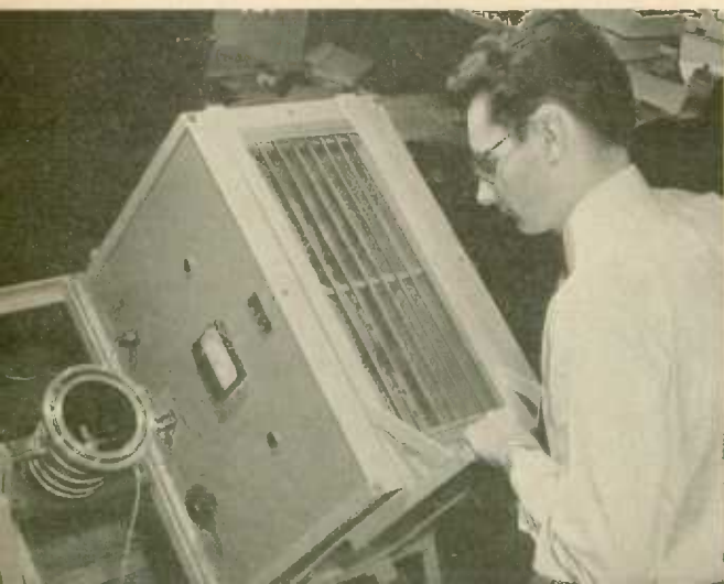
An induction melting and casting unit in which small samples of high purity metals may be melted and chill-cast in a vacuum or preferred atmosphere.
