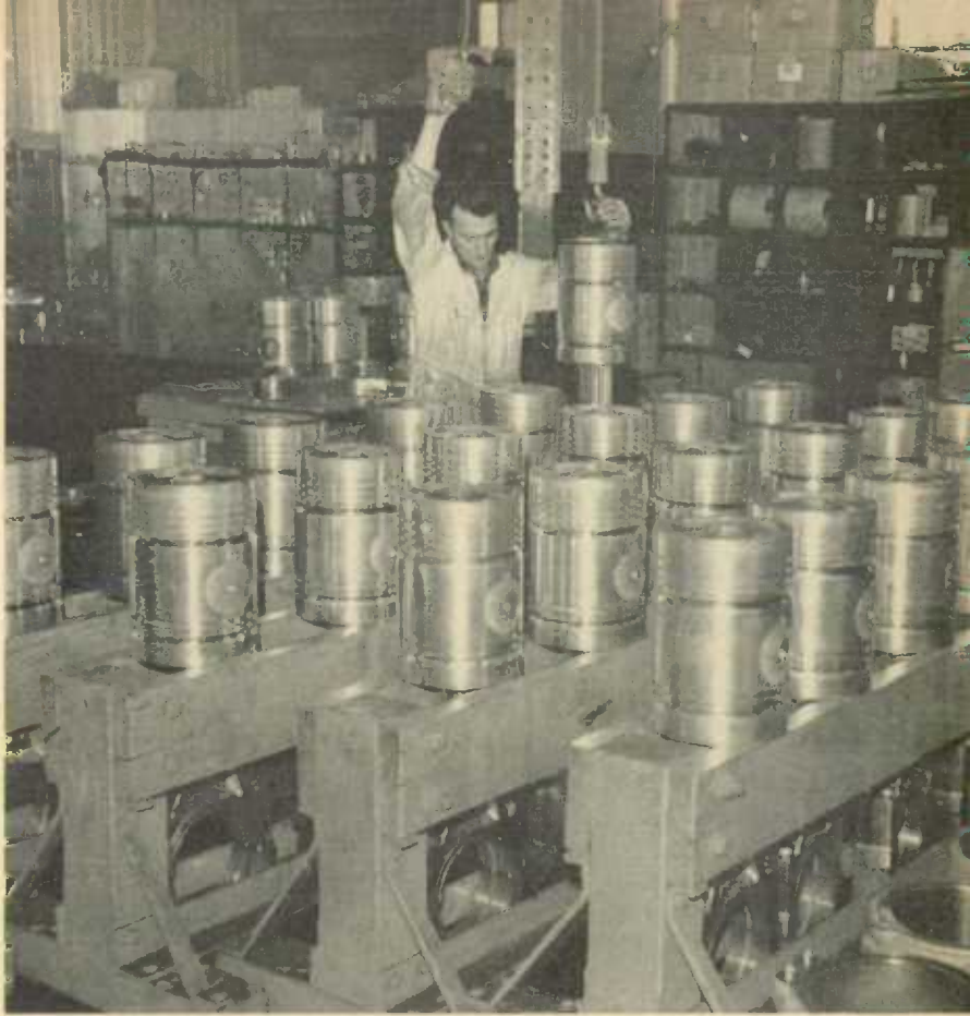
Pistons being assembled to connecting rod for installing into a diesel engine.
