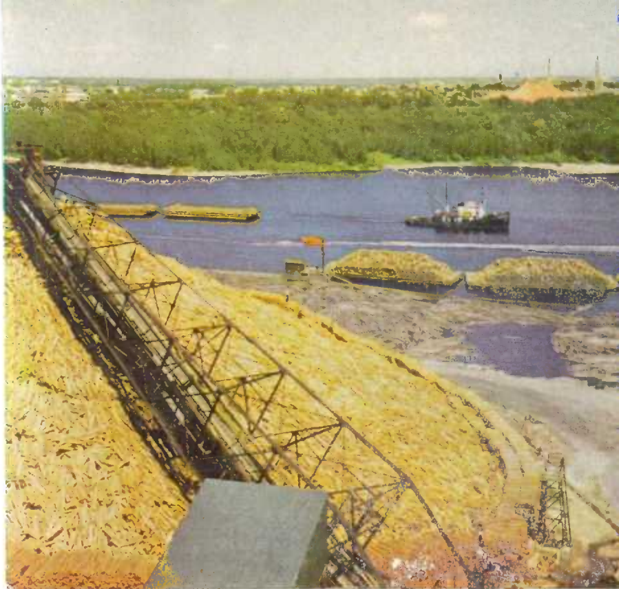
Pulpwood from the Gatineau and Ottawa River forests—raw material for an integrated mill producing newsprint, dissolving and paper pulps and various building boards. The dissolving wood cellulose is used in the manufacture of rayon, cellophane and other plastics, bleached sulphite emerges as bond paper and the sugar content of the waste liqueurs of the sulphite pulping process is recovered and refined into ethyl alcohol.
