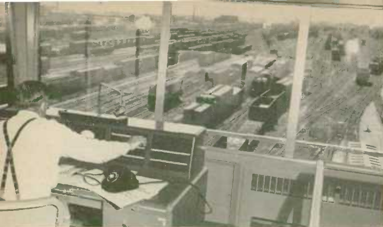
A yardmaster surveys freight operations from his seven-storey vantage point. A two-way loud speaker system keeps him in touch with switching crews on the ground.
