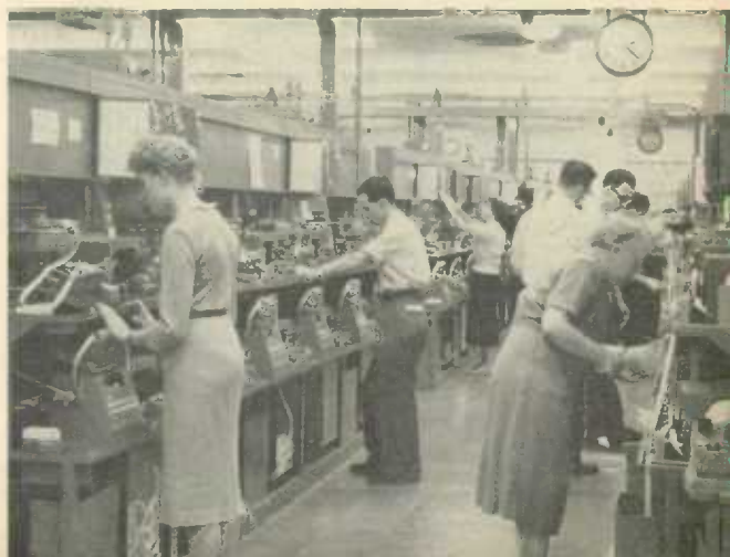
This collection of teletypes, flashing lights and control boards in Montreal's Bonaventure Terminal is busy 24 hours a day transmitting and receiving messages to and from the entire world. It can handle 82,000 messages a day and is one of the most efficient methods of transmission ever devised.
