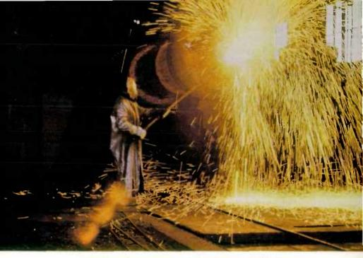
A skilled steelmaker uses an oxygen torch to strip the scale off a forging.
