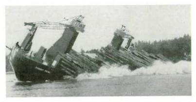
A self-dumping barge carrying 1,000,000 board feet of spruce and cedar discharges its cargo in three to four seconds on arrival at the booming grounds. Advantages over transport by deep-sea raft are that barges can be towed faster, there is less danger of losing logs in a storm and, since the logs spend less time in salt water, damage from insects is reduced.
