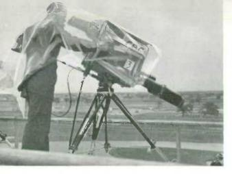
A CBC technician and a camera share the latest in transparent rain wear—a plastic hood designed to protect man and machine from bad weather during telecasting of outdoor events. Nearly 1,000 skilled technicians maintain and operate cameras and other electronic equipment in CBC's 18 production centres across Canado and hundreds are employed in private television stations.
