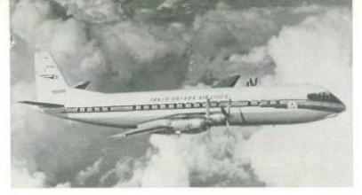
The new propeller-turbine Vanguard made its first scheduled run on January 31, 1961. This 96-passenger, 425-m.p.h. airliner is used on short to medium-range routes in Canada, to the United States and south to Bermuda and the islands of the Caribbean.
