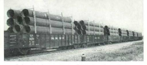
The first carloads of steel pipes shipped out of the tube plant at Camrose, Alberta, following completion of a \$3,000,000 extension program. These big pipes will be used in the construction of ail and gas pipelines.
