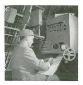
Meteorological research is impartant in transport, communications, agriculture and other fields. In the dome of the weather station building at Maniwaki, Quebec, a technician tracks down a balloon and radiosonde transmitter by radio direction finder, thus recording direction and velocity of the wind at upper air levels.
