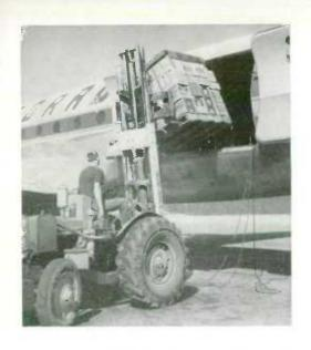
"Palletizing", or the strapping of loads of freight to pallets which are then farklifted into aircraft, has vastly speeded spacetions at both ends of the flight.
