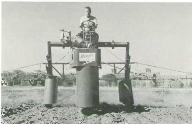
A self-propelled sprayer that can be raised to six feet for corn or lowered to six inches for strawberries.
