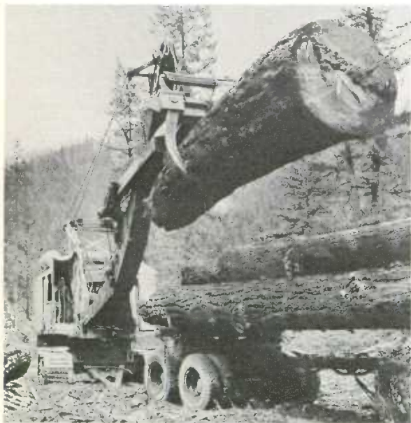
This fabulous machine for loading the enormous logs from the British Columbia forests onto trailers is nicknamed the "cherry-picker".
