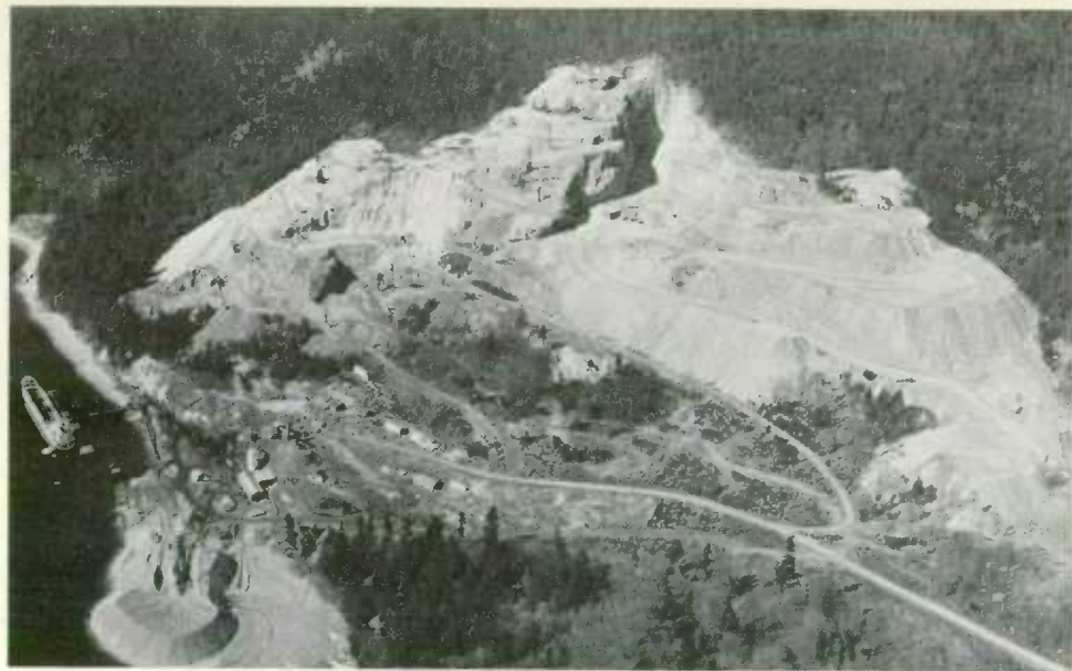
The large open pits from which iron ore is derived on Texada Island, British Columbia, and the 2,500-ton mill in which concentrates are produced. In this photograph a Japanese freighter is seen loading magnetite for shipment to Japan.
