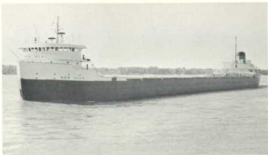
One of the newest additions to the Great Lakes fleet, the Red Wing , with a length of 730 feet and a beam of 75 feet, is the largest ship that can be accommodated through the locks on the St. Lawrence Seaway.
