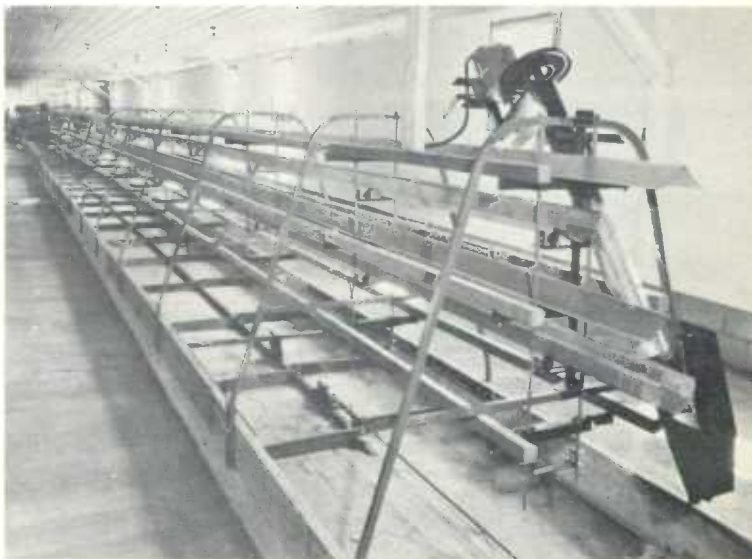
Automatic feeding, watering and manure-disposal unit in a modern poultry house.
