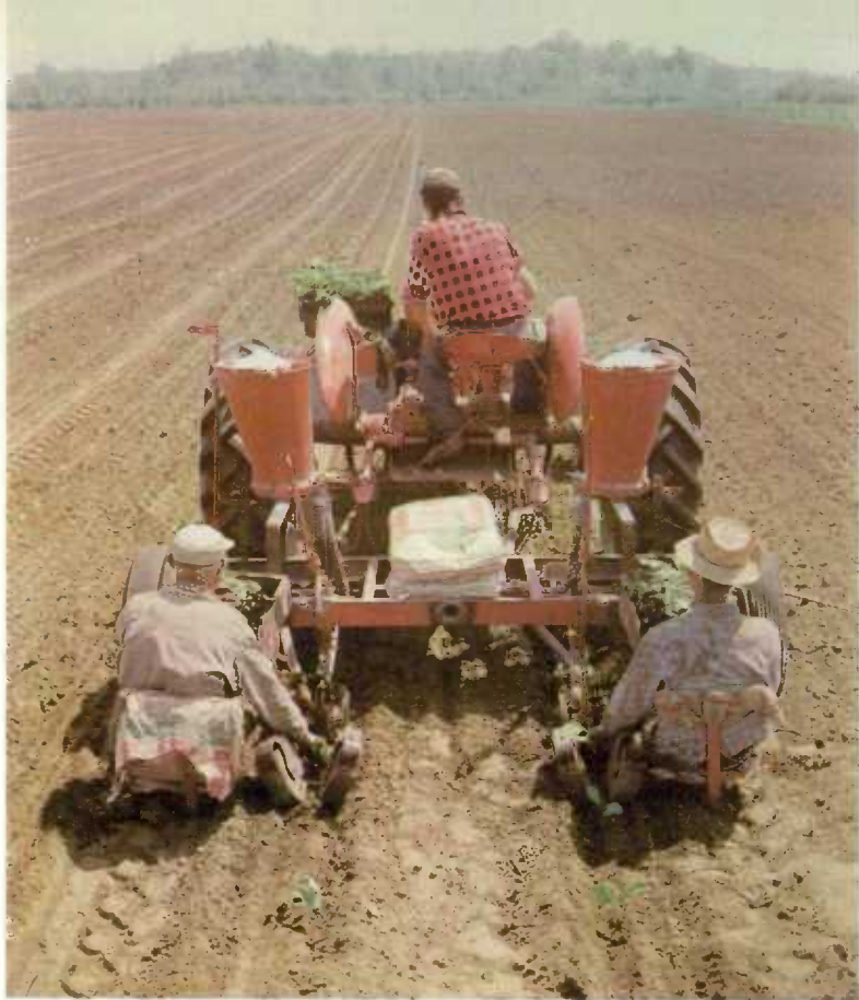
This tractor-driven transplanting rig deposits fertilizer on both sides of shallow trenches approximately 40" apart. Every two feet it releases a jet of water, at which point the men seated behind the tractor place the transplants in the trench. It is then closed in by two metal arms. In this picture, tobacco plants are being set out.
