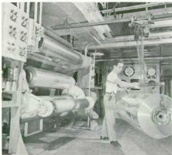
Synthetic materials play an important part in the packaging so widely accepted today. Here a completed roll of cellulose film is swung away from the wind-up end of a casting machine.
