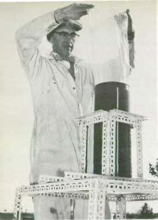
Fallout from the skies is checked by testing daily air samples collected at meteorological stations across Canada. Rain and snow samples fall into plastic bags which are changed every month and sent to the Department of National Health and Welfare for analysis.
