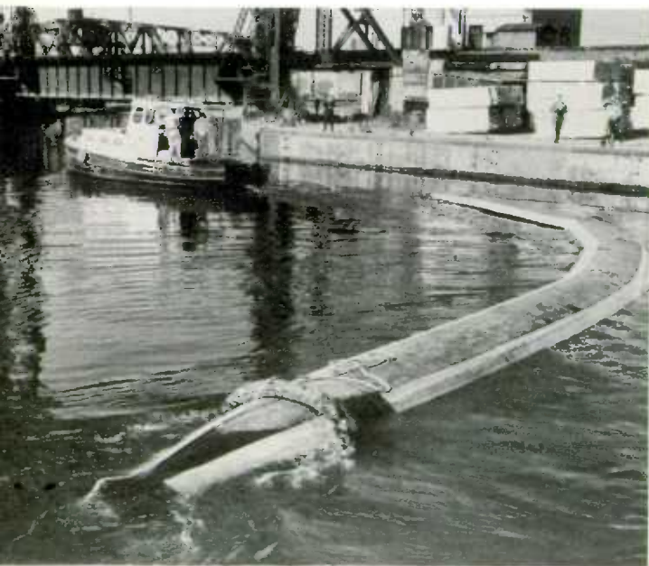
Flexible, towable containers, with capacities ranging from 15 to 320 tons, are used extensively for carrying petroleum products. During the summer of 1961, the Department of Transport tested these units in the Arctic where difficulties often exist in bringing oil into shore because of shallow water.
