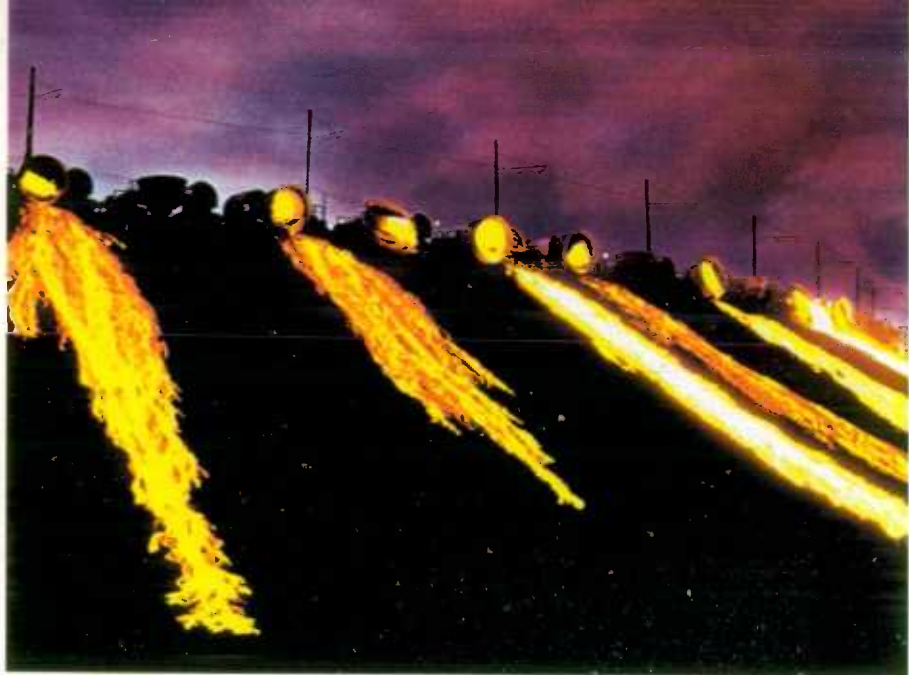
Pauring slag at night at International Nickel's operations at Copper Cliff, Ontario. Slag trains, powered with two electric locomotives, run approximately every half hour and consist of 18 slag cars carrying 16-ton-capacity slag pots. Molten slag is dumped by rotating the pots on each slag car.
