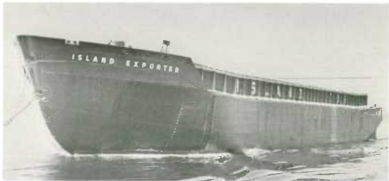
What is claimed to be the world's largest deep sea deck cargo barge was built at Esquimalt, B.C. to carry crushed limerock from Blubber Bay in the Gulf of Georgia to Lake Oswego, Oregon. The barge has a capacity of 10,700 tons, yet can negotiate the 20-foot-deep, 200-foot-wide channel of the Willamette River.
