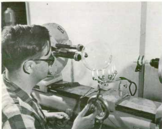
A glass-blowing lathe, which automatically turns and mechanically blows glass, in use at the National Research Council laboratory in Halifax.
