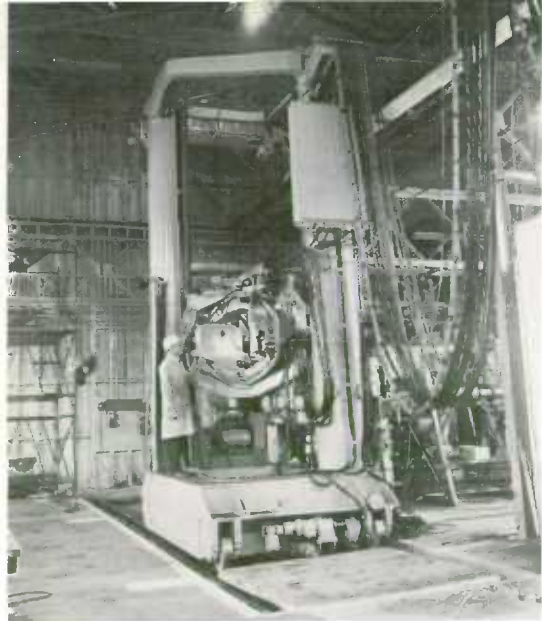
Testing one of the two fuelling machines for the Douglas Point Nuclear Power Station. Used fuel will be removed and new fuel will be inserted in the reactor without shutting down the plant.
