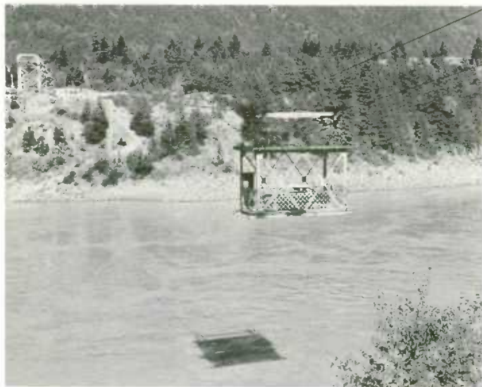
An unusual mode of transportation — an aerial car ferry that carries pedestrians and one car across the Fraser River between Boston Bar and North Bend, B.C. It can carry up to three tons, operates 24 hours a day and is free.
