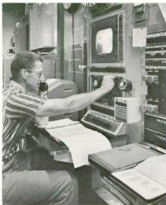
Every TV station in Canada is associated with a telephone company television operating centre. Technicians monitor the transmissions, switch programs, test and line up the microwave facilities.
