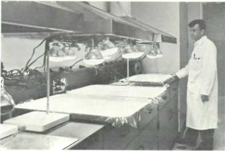
Infra-red lamps are used to evaporate samples of water which will be tested for radioactive fallout components. This is part of the program conducted by the Radiation Protection Division of the Department of National Health and Welfare.
