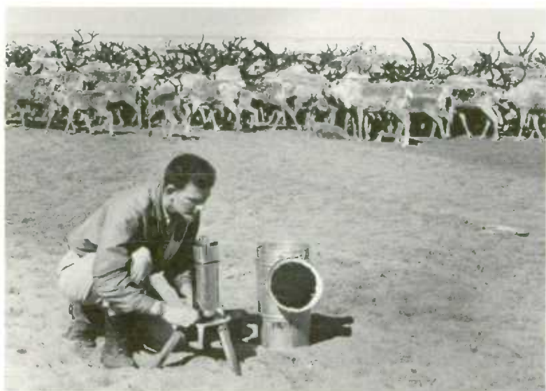
A herd of reindeer in the Mackenzie Delta, north of the Arctic Circle, is undisturbed by a geophysical observer who is reading a gravity meter, during an evaluation of potential petroleum resources of the region.
