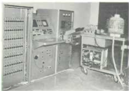
An electric model heart, designed to reproduce all the electrical activity of the normal heart, was designed for study at the National Research Council. It is shown at the right, with recording equipment to the left.
