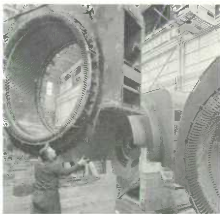
These 6,500-horsepower synchronous motors manufactured in Hamilton, Ontario, are prepared for export to an oil refinery in Greece.
