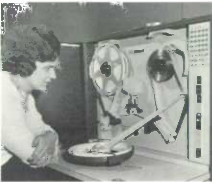
All income tax returns of Canadians are processed at the Department of National Revenue Taxation Data Centre. Information from returns is key-punched onto paper tapes, double-checked, then transferred to magnetic tapes for "memory storage" and feeding into the electric computer. One reel of magnetic tape can hold tax data on 100,000 Canadians.
