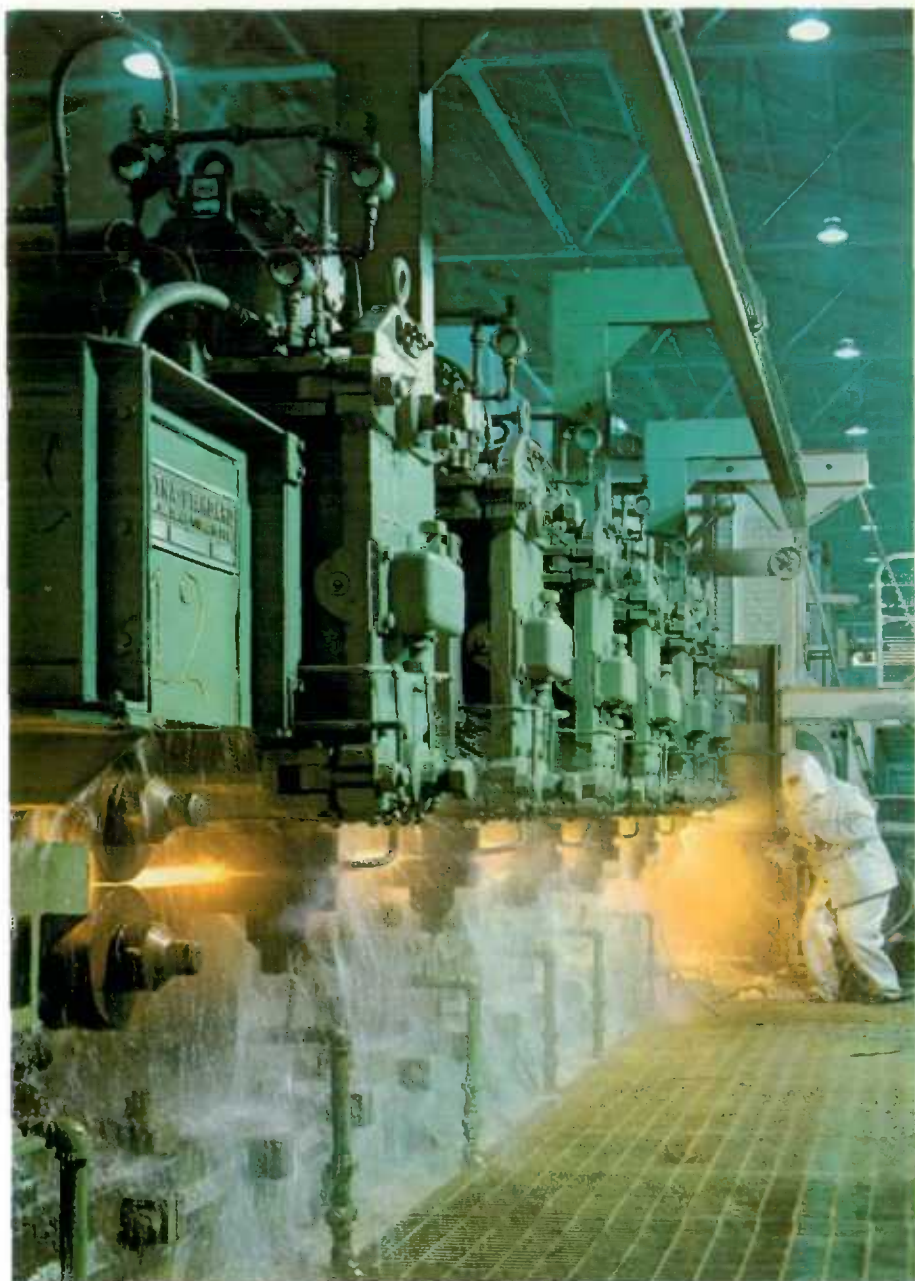
A continuous butt-welding pipe mill at the Steel Company of Canada, Limited, McMaster works, Contrecoeur, Quebec.
