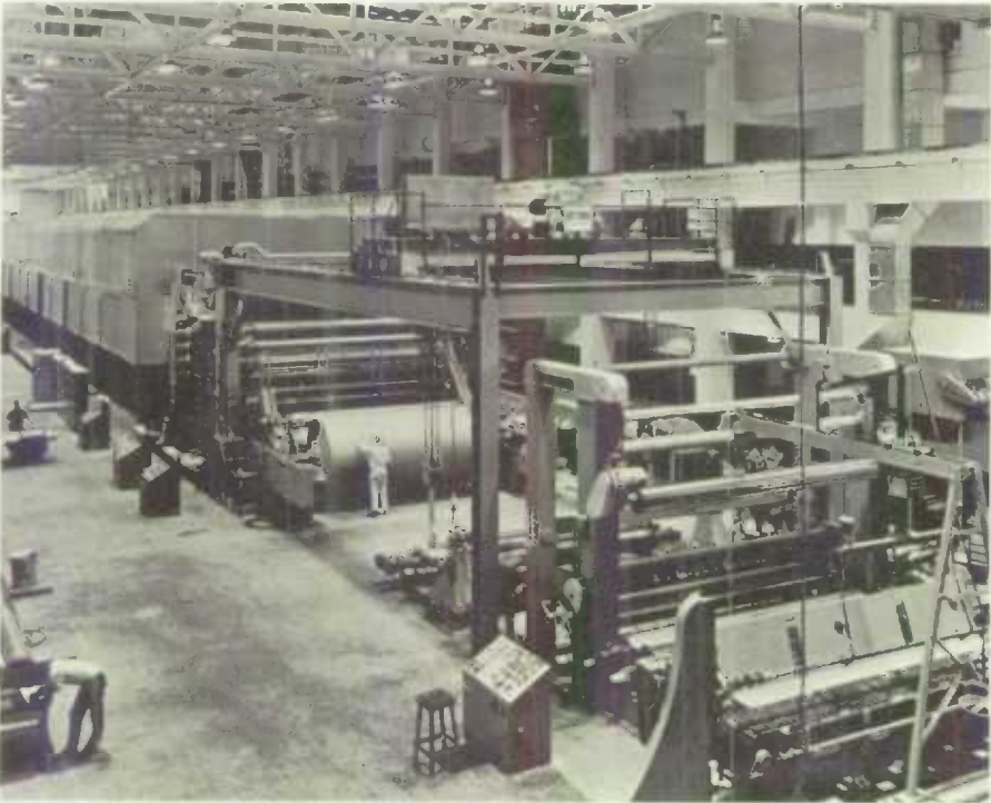
A kraft specialty machine at Crown Zellerbach's Elk Falls plant can produce stretchable paper, useful for packaging fertilizer and cement.
