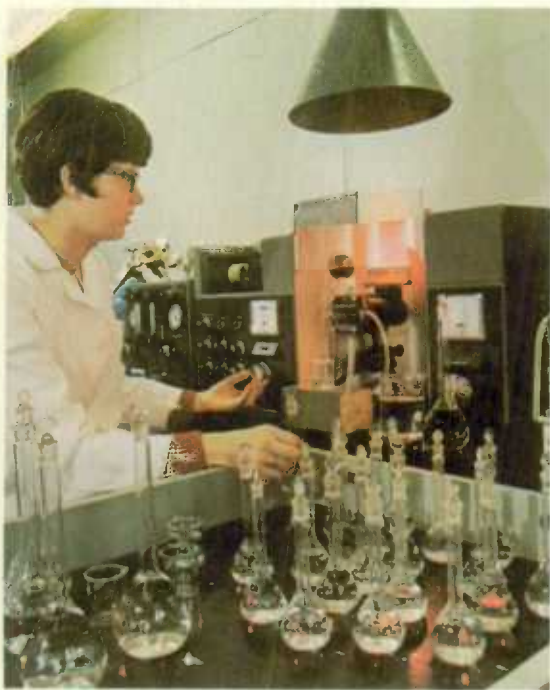
The atomic absorption spectrophotometer is used in the Mines Branch of the Department of Energy, Mines and Resources to determine the various elements in sample rocks in solution.
