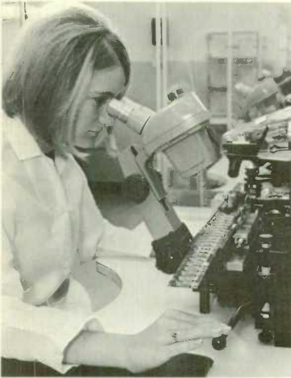
A technician works with microscope and semi-automatic equipment to weld minute strands of gold wire to interconnect package posts and ohmic metal patterns on the circuit.
