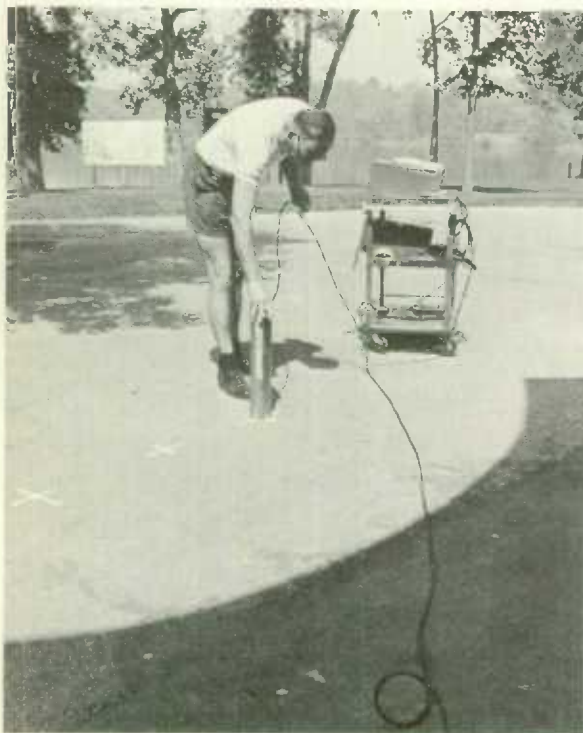
A technician in the Radiation Protection Division of the federal Health and Welfare places a sensor on a pre-determined grid to test the course of effluent from public washrooms in order to detect defects that might permit contamination of nearby Leamy Lake, Que.
