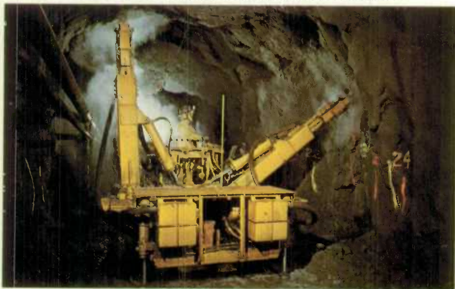
Modern drill jumbo is employed in the Craigmont Mines, Merritt, B.C.
