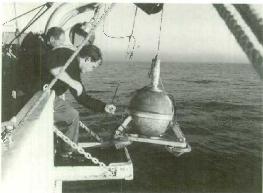
A gravimeter is lowered to the floor of Hudson Bay to take spot measurements of the pull of gravity on the bottom.
