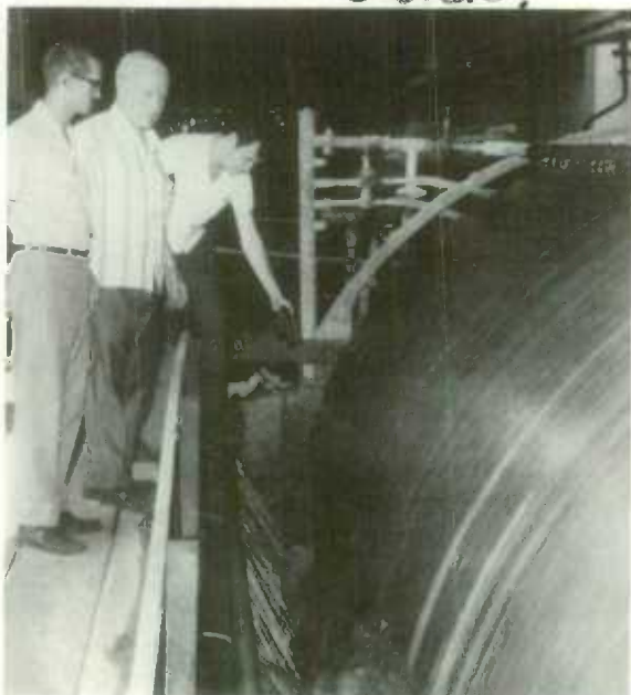
Near Nova Lima, Brazil, a CESO volunteer and the local chemist and metallurgist check the operation of a tailing filter to recover minerals being lost.
