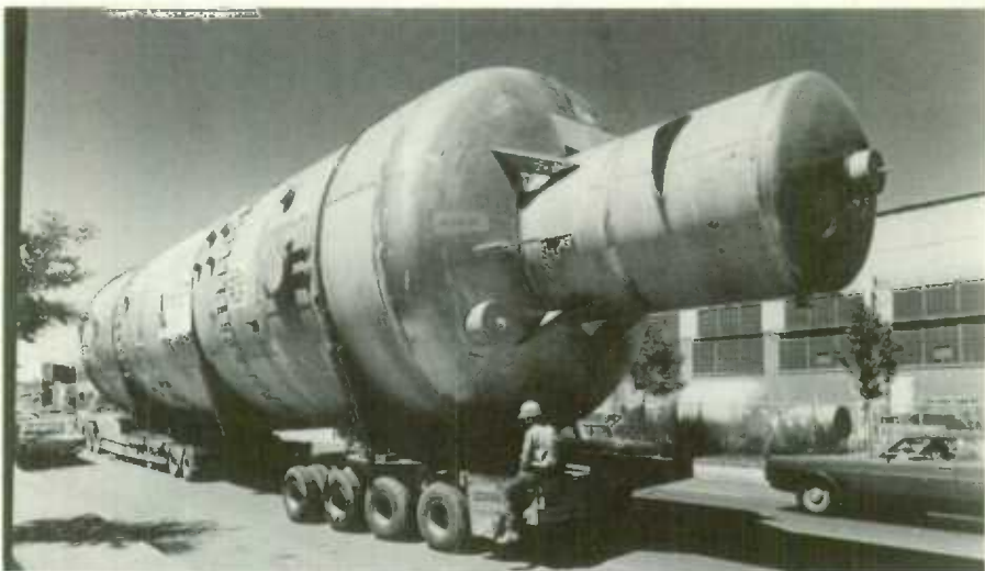
One of 17 distillation columns each weighing 60 tons is on its way from Montreal, Que., to Texas. It is used to separate liquid oxygen from atmospheric air at -320^{\circ}\text{F} .
