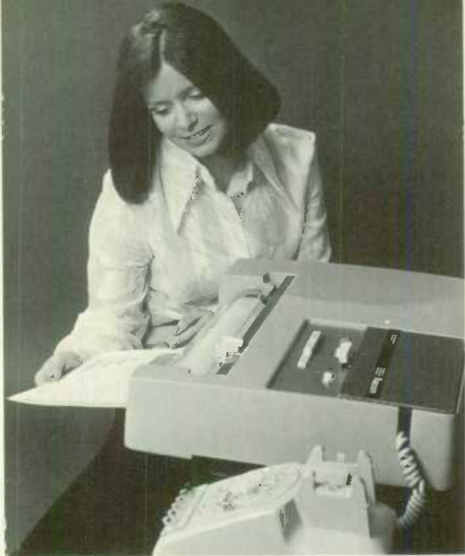
A recently introduced facsimile terminal service called Faxcom, when coupled to a telephone handset, can send a page of words or pictures over telephone lines.
