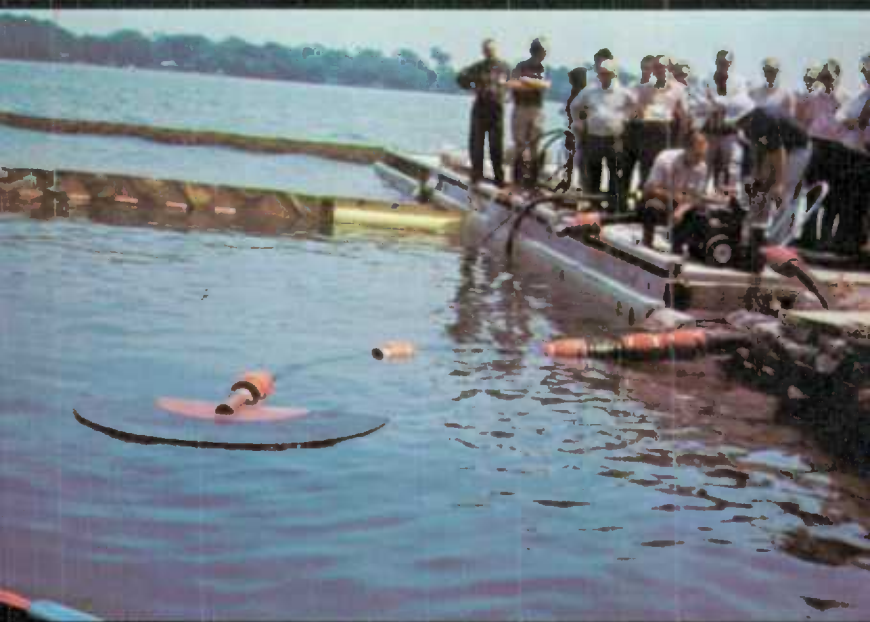
The skimming head in the foreground, the boom in the background, and other oil-spill equipment are transported by mobile vans to strategic locations.
