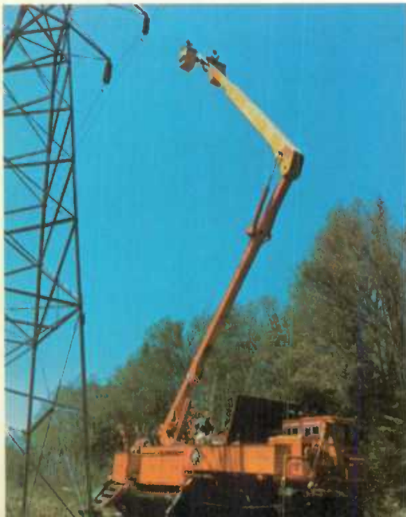
A 29-ton Ontario Hydro vehicle lifts linemen in insulated buckets up to 75 feet in the air to work on "live" 500,000 volt lines.
