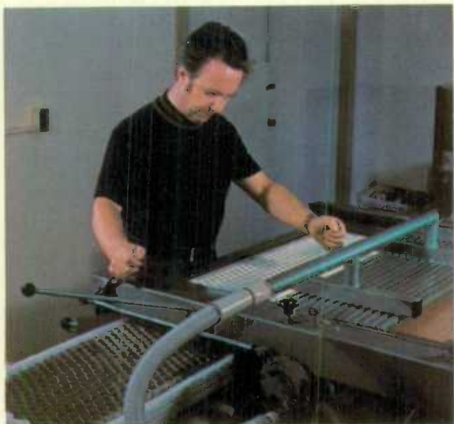
Containerized planting is becoming an integral part of reforestation. The Forestry Service is testing this machine which is capable of loading 50,000 paper-pot seed containers per hour.
