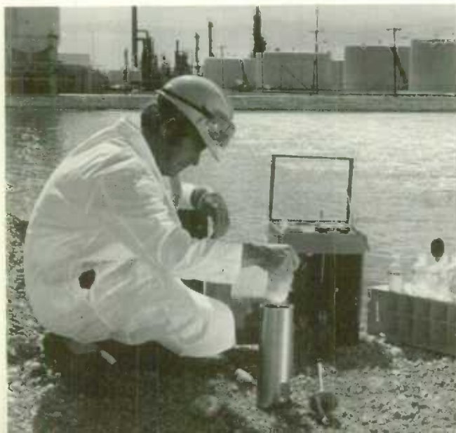
The $400,000 biochemical lagoon undergoes tests at Imperial Oil's Winnipeg refinery. Waste water is treated in the lagoon before discharge into the Red River nearby.
