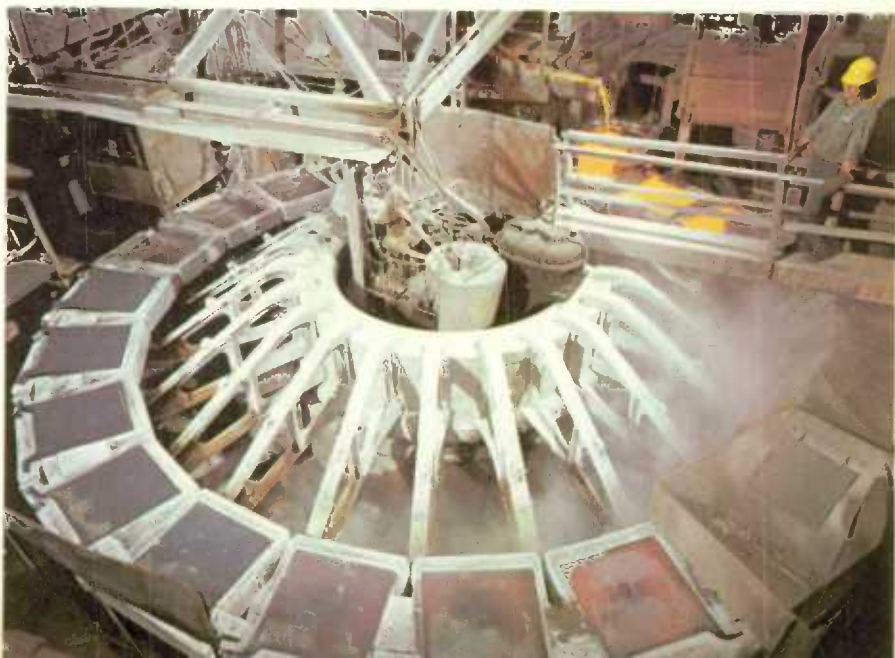
Copper anode casting wheel at Noranda's copper smelter in Quebec.
