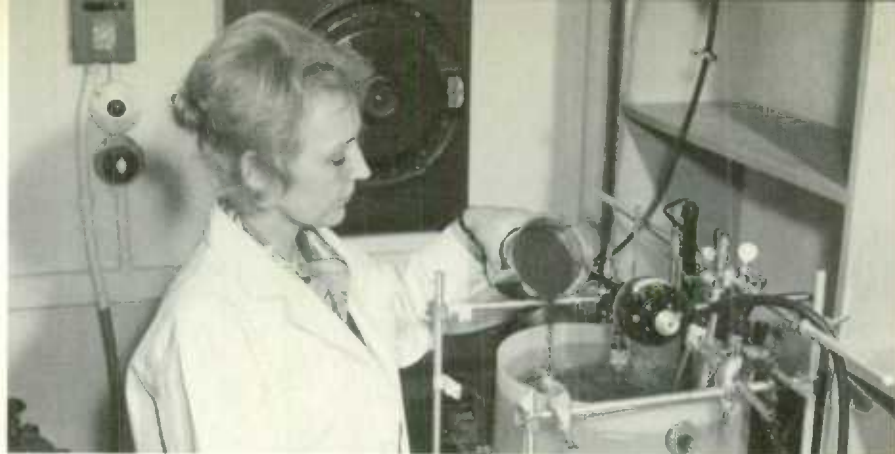
A method of removing toxic substances from rapeseed has been discovered at the University of Saskatchewan. Dr. Kozłowska, co-worker on the study, is feeding rapeseed into a water solution to study conditions under which toxic materials are removed from intact seeds.
