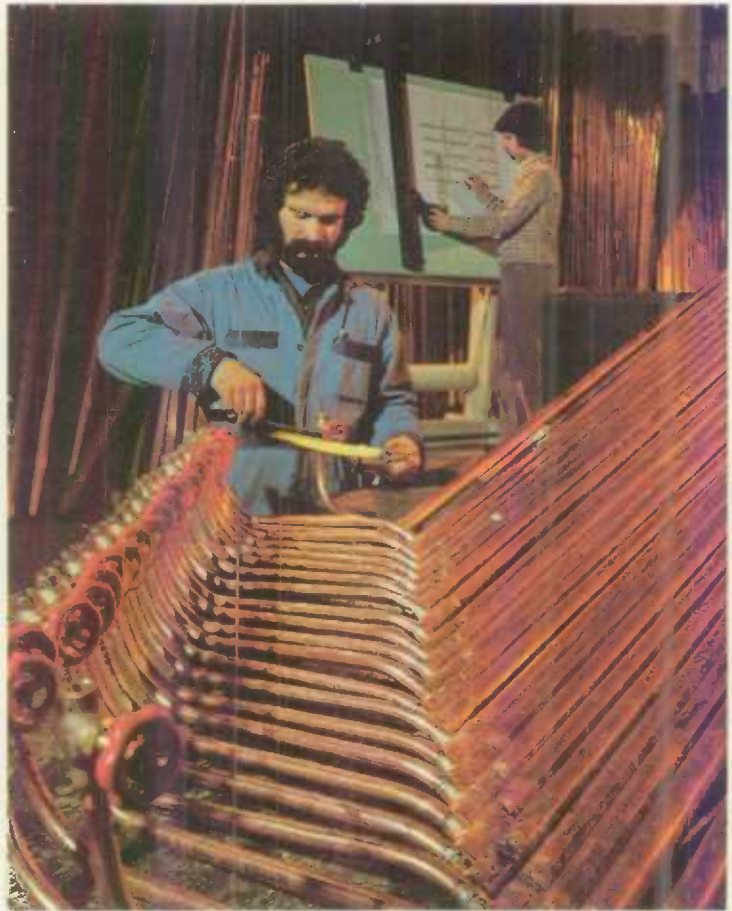
Welding pipes for heating and plumbing installations in apartments and commercial buildings.
