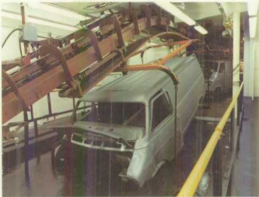
Van bodies are completely immersed and coated with primer at the Chrysler Canada Ltd. plant in Windsor, Ont.
