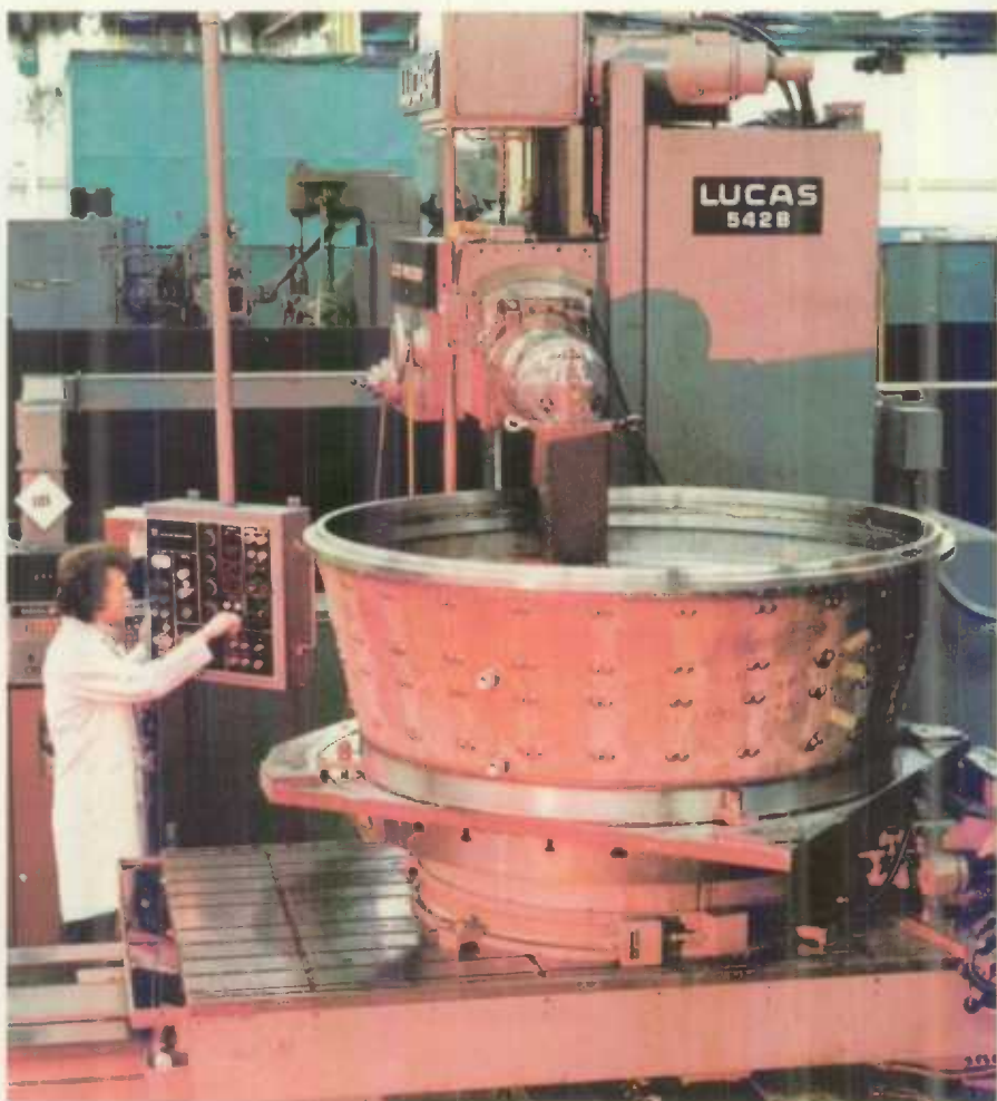
An industrial gas turbine casting being machined at a plant in Mississauga, Ont.
