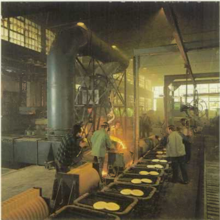
Pouring metal into shell moulds at the ductile iron foundry in Welland, Ont.
