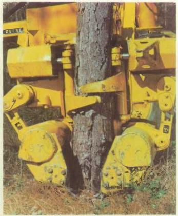
A tree shear clamps on to a tree trunk while its curved blades cut the tree near the ground with a minimum of waste and damage.
