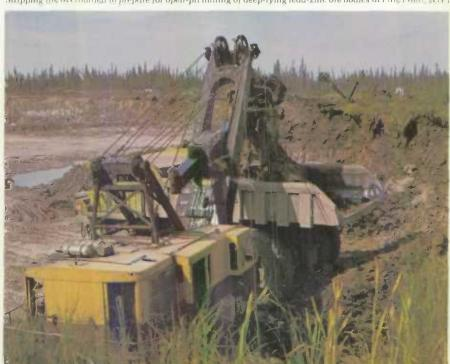
Stripping the overburden to prepare for open-pit mining of deep-lying lead-zinc ore bodies at Ping Point, NWT.
