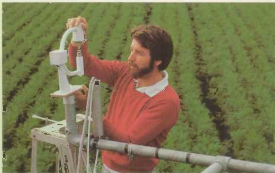
A monitoring instrument, installed by Ontario Hydro, determines the dry deposition rates of acid gases in an acid rain research program.
