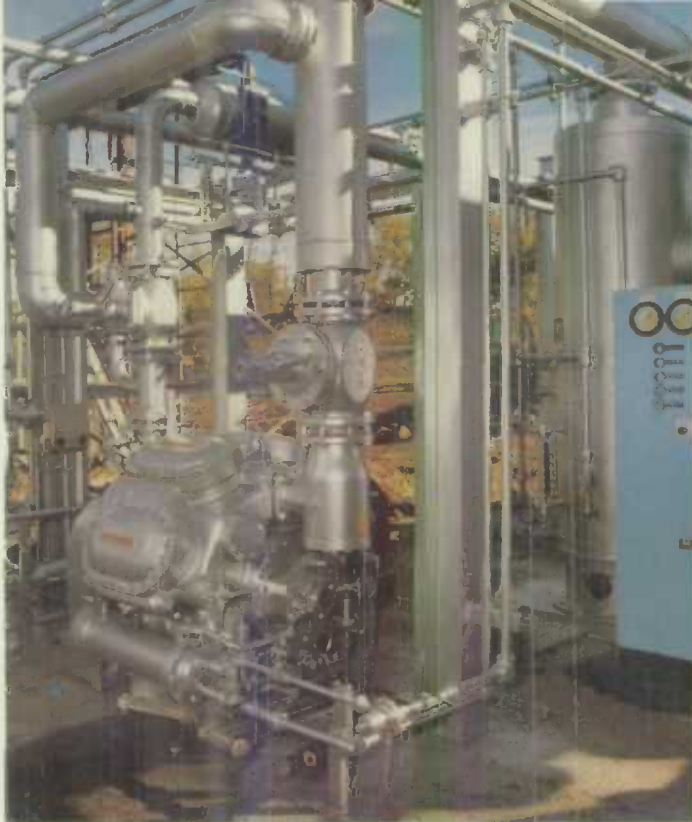
Propane refrigeration compressor at Mikwan Gas Plant in Alberta. The compressed propane is used to produce refrigeration to remove liquid hydrocarbons from natural gas to make the gas suitable for home heating.
