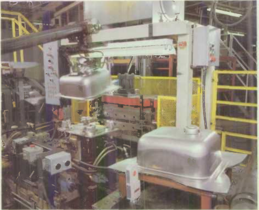
Robotic arm loads and unloads hydraulic press that produces stainless steel kitchen sinks.
