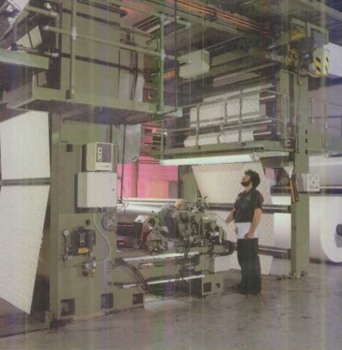
Printing enter coating for corrugated containers at high-tech paper converting plant at Mississauga, Ont.
