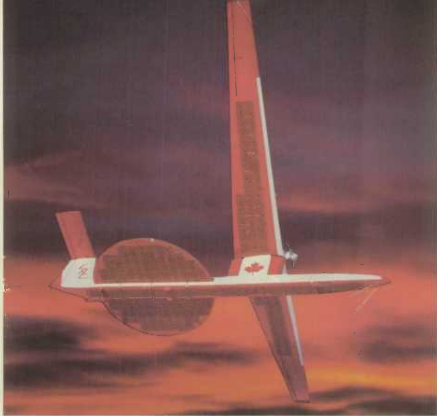
SHARP (Stationary High Altitude Relay Platform) — the world's first microwave-powered aircraft capable of uninter-rupted flight. A current focus of research efforts is on designing a small pilot-less microwave-powered aircraft to serve as an inexpensive alternative to a satellite.
