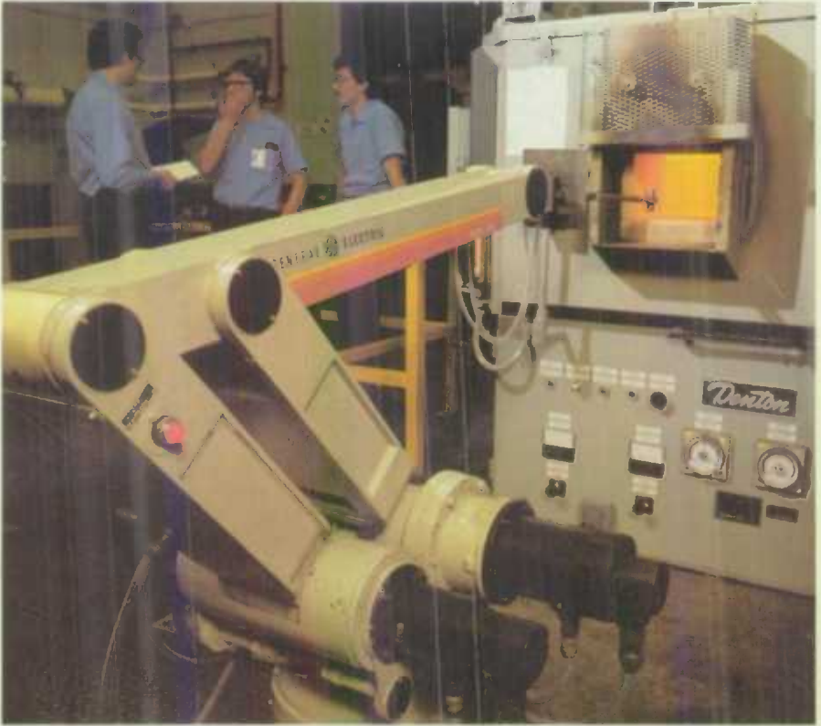
Robotic arm lifts metal cylinder from heat treating furnace at an auto engine plant in Quebec.
