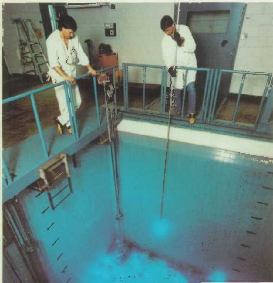
Storing cobalt-60 at Nordion. Cobalt-60 is the radioactive element used in the cobalt machines which treat cancer.
