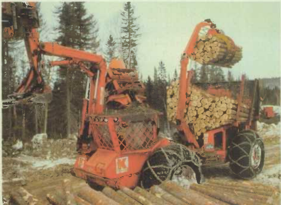
Tree harvester transferring logs onto storage pile in the Mont Tremblant area of Quebec.
