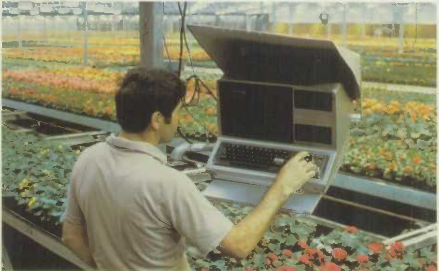
A computer controls the light, temperature and humidity in a greenhouse at Campbellvale, Ont.
