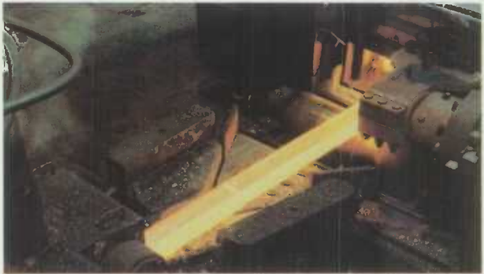
Steel billets leaving the reheating furnace to be rolled into wire rod at a rolling mill operation in L'Orignal, Ont.
