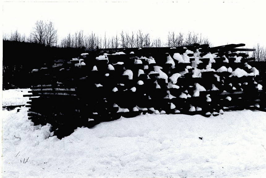
Untrimmed 2-inch Rough Dimension Lumber Stripped for Air-drying at Waterhen Lake (Old Sawmill Site)
