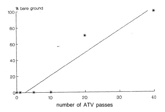
FIGURE 5: Regression plot of amount of bare ground and the number of ATV passes for the test plot.
