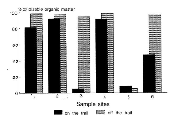
FIGURE 2: Results of loss of weight on ignition tests on the lake trail.
